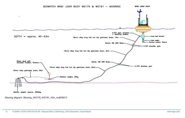
Figure 2. Illustration of a meteorological buoy and mooring configuration (Vineyard Wind SAP 2020); Vineyard Wind may deploy up to two of buoys at areas SAP-1 and SAP-2.
