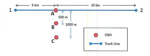
FIGURE 4. AMAR recorder deployment geometry relative to vessel sail track for support vessel sound characterization measurements.
