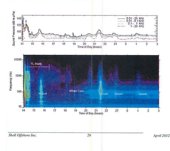
Figure 5. Lower: spectrogram of sound level measurements obtained from a hydrophone recording system. Upper: broadband and selected band level variation with time.
