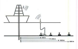
FIGURE 2. Geometry of the real-time telemetered acoustic system and three autonomous acoustic recorders that will sample sound produced by drilling operations of drillship *Kulluk*
