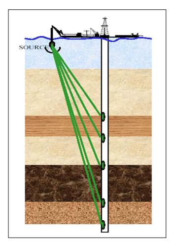
Figure 1-2 Schematic of ZVSP
