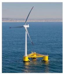
Full-scale prototype of WindFloat device
