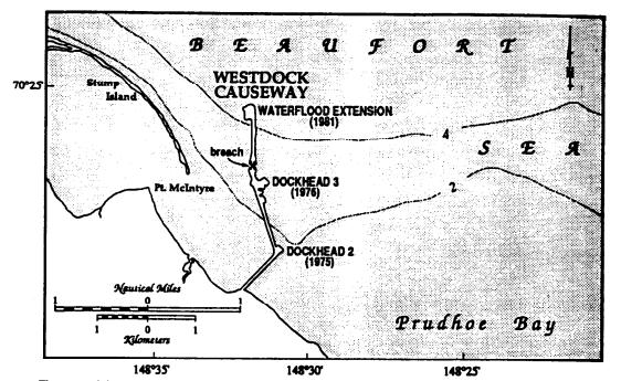
Figure 2. West Dock causeway, showing sequential extensions (depths in meters).
