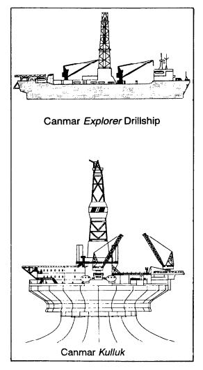
Figure 1. Canmar *Explorer* Drillship and *Kulluk* Floating Drilling Unit.
