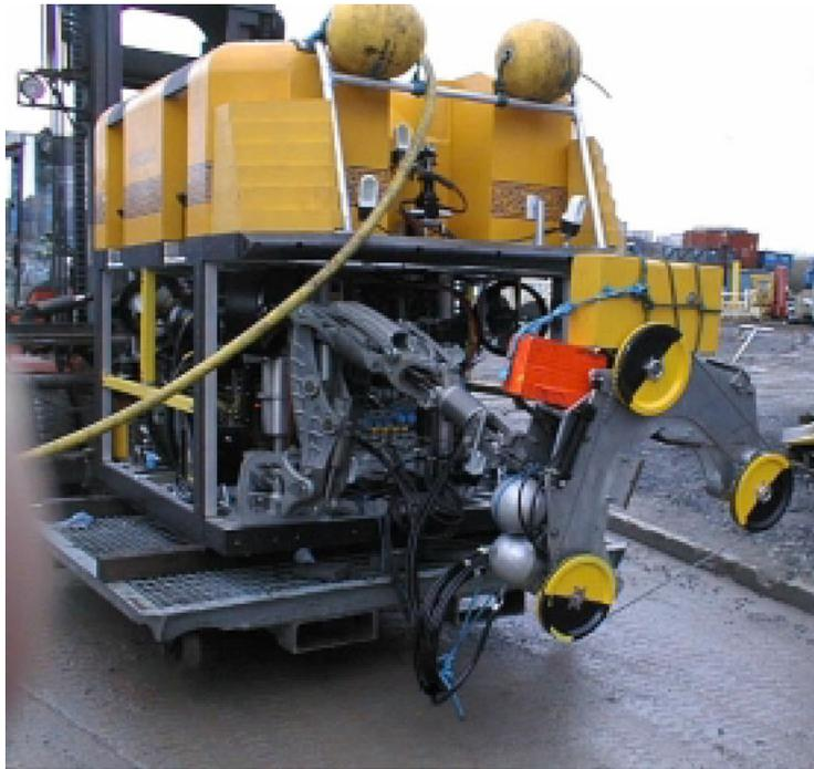
Figure 6.5. Diamond Wire Cutting System Deployed from an ROV for Use in Pipeline or Small Member Cutting (Courtesy of CUT USA, Inc.).
