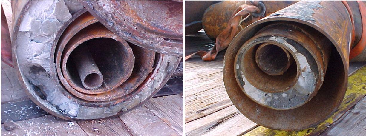
Figure 3.2. Partially Grouted Conductors with Eccentric Casing Strings.
