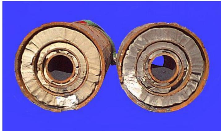
Figure 3.1. Grouted Conductor Cross-section with Concentric Casing Strings.
