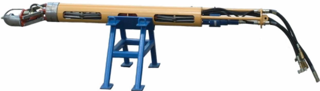
Figure 6.3. Abrasive Water Jet Cutting Tool for Conductors or Small Piles (Courtesy of Circle Technical Services).
