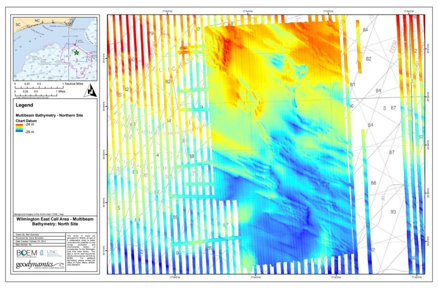
Figure 3-12. Map displaying bathymetry at the full coverage area referred to as the "north" site, overlaid on the "overview" bathymetry.
