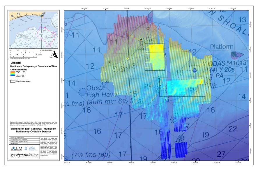
Figure 3-11. Results of the "overview" multibeam bathymetry dataset with the "sites" overlaid and labelled for reference.
