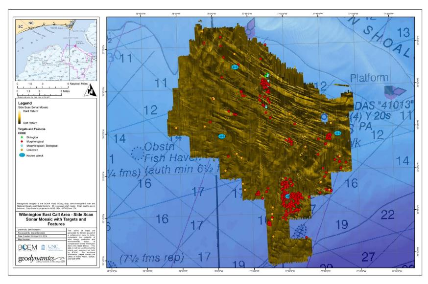
Figure 3-4. Results of the sidescan sonar target and feature database, overlaid on the sidescan sonar mosaic.
