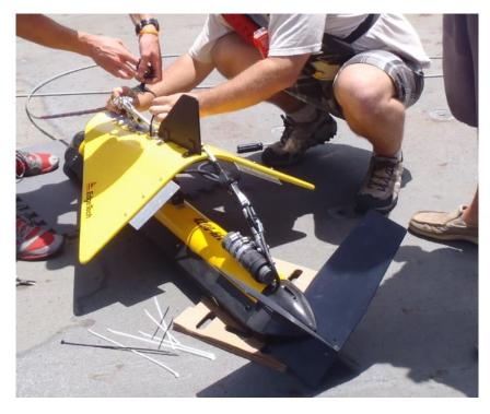
Figure 2-4. Picture of the Edgetech towfish used to collect sidescan sonar data.
