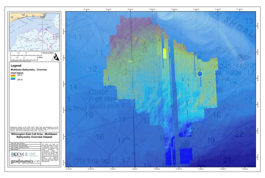
Figure 3-10. Results of the multibeam bathymetry dataset referred to as the "overview" data.
