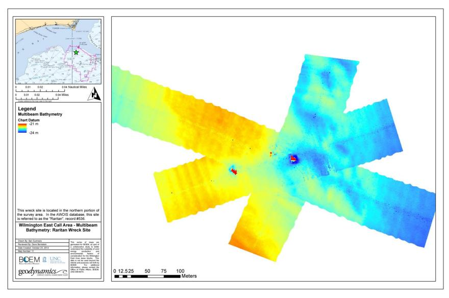
Figure 3-14. Map displaying bathymetry over the AWOIS wreck site referred to as the "Raritan".
