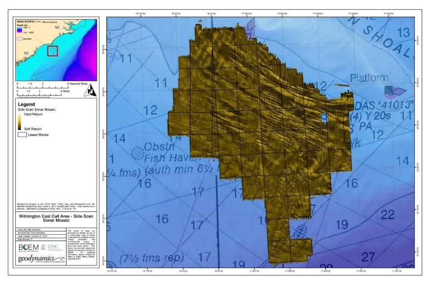
Figure 3-3. Results of the sidescan sonar mosaic, overlaid by OCS lease blocks.
