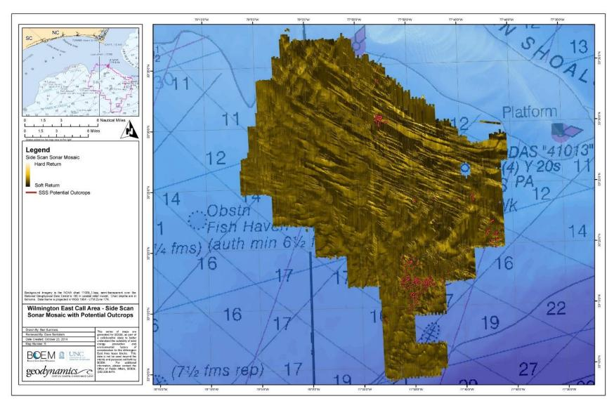
Figure 3-5. Results of the digitized potential outcrops, overlaid on the sidescan sonar mosaic.
