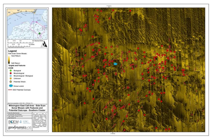
Figure 3-7. A zoomed in view of a cluster of features identified in the southern part of the survey area, overlaid by digitized outcrops.
