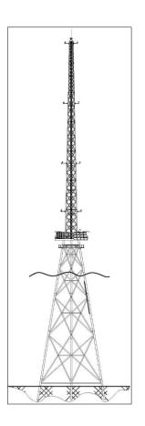
Figure 3-3(a) Lattice-Type Mast-Mounted Meteorological Tower on a Monopile Foundation
