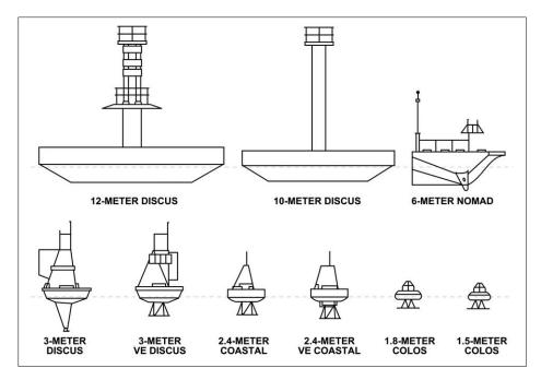
Figure 3-4 Buoy Schematic Source: National Data Buoy Center, 2008
