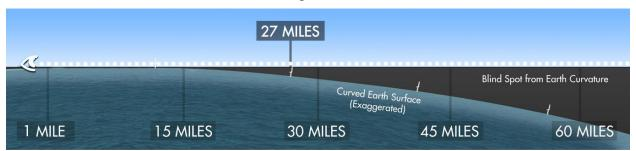
Figure 4-24 Distance at Which the Proposed Meteorological Tower Would Drop Below the Horizon Based on a Height of 394 ft (120 m)
