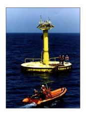
Figure 3-5(a) 10-Meter Discus-Shaped Hull Buoy
