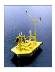
Figure 3-5(b) 6-Meter Boat-Shaped Hull Buoy
