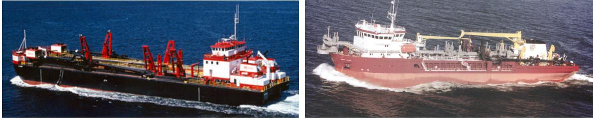
Figure 2. Manson's Bayport Hopper Dredge (left) and Great Lakes Hopper Dredge Liberty Island (right) (Courtesy of Manson Construction and Great Lakes Dredge & Dock)
