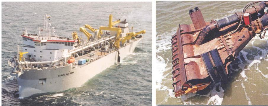
Figure 1. Jen de Nul's Vasco de Gama (left) and Typical Draghead (right) (Courtesy of Jen de Nul)
