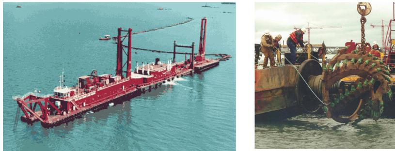
Figure 4. Great Lakes Cutter Suction Dredge California (left) and CutterHead (right) (Courtesy of Great Lakes Dredge & Dock)
