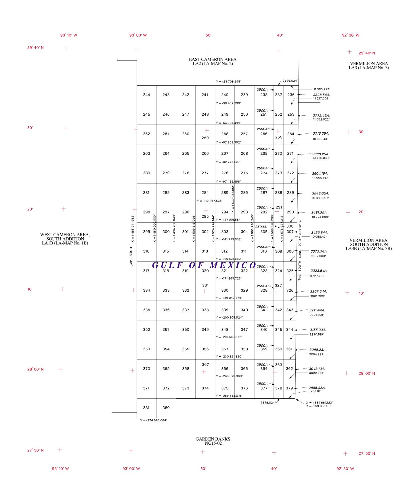
All blocks are based on the Louisiana (Lambert) Plane Coordinate System, South Zone, with X origin = 2,000,000' at  $91^{\circ} 20'$  W and Y origin = 0.00' at  $28^{\circ} 40'$  N.
