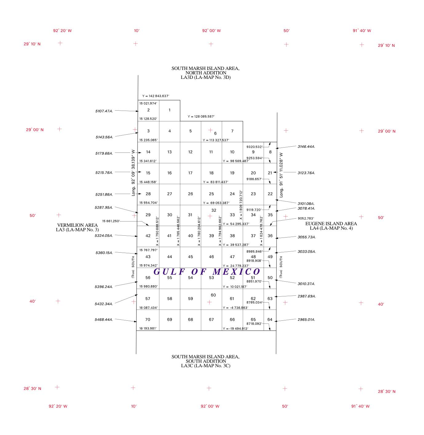
All blocks are based on the Louisiana (Lambert) Plane Coordinate System, South Zone, with X origin = 2,000,000' at  $91 \degree 20'$  W and Y origin = 0.00' at  $28 \degree 40'$  N.
