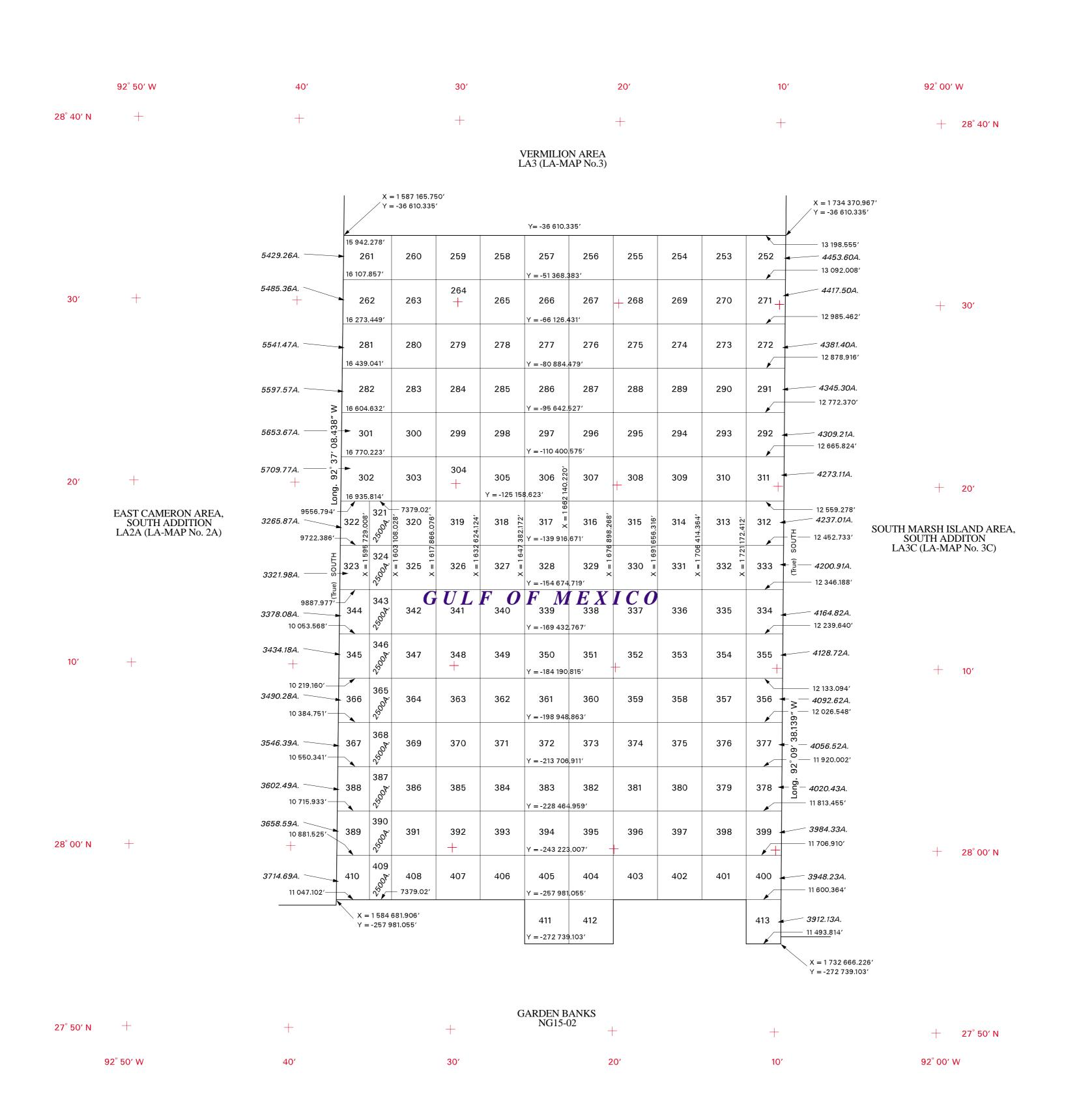
All blocks are based on the Louisiana (Lambert) Plane Coordinate System, South Zone, with X origin = 2,000,000' at  $91^{\circ} 20'$  W and Y origin = 0.00' at  $28^{\circ} 40'$  N.
