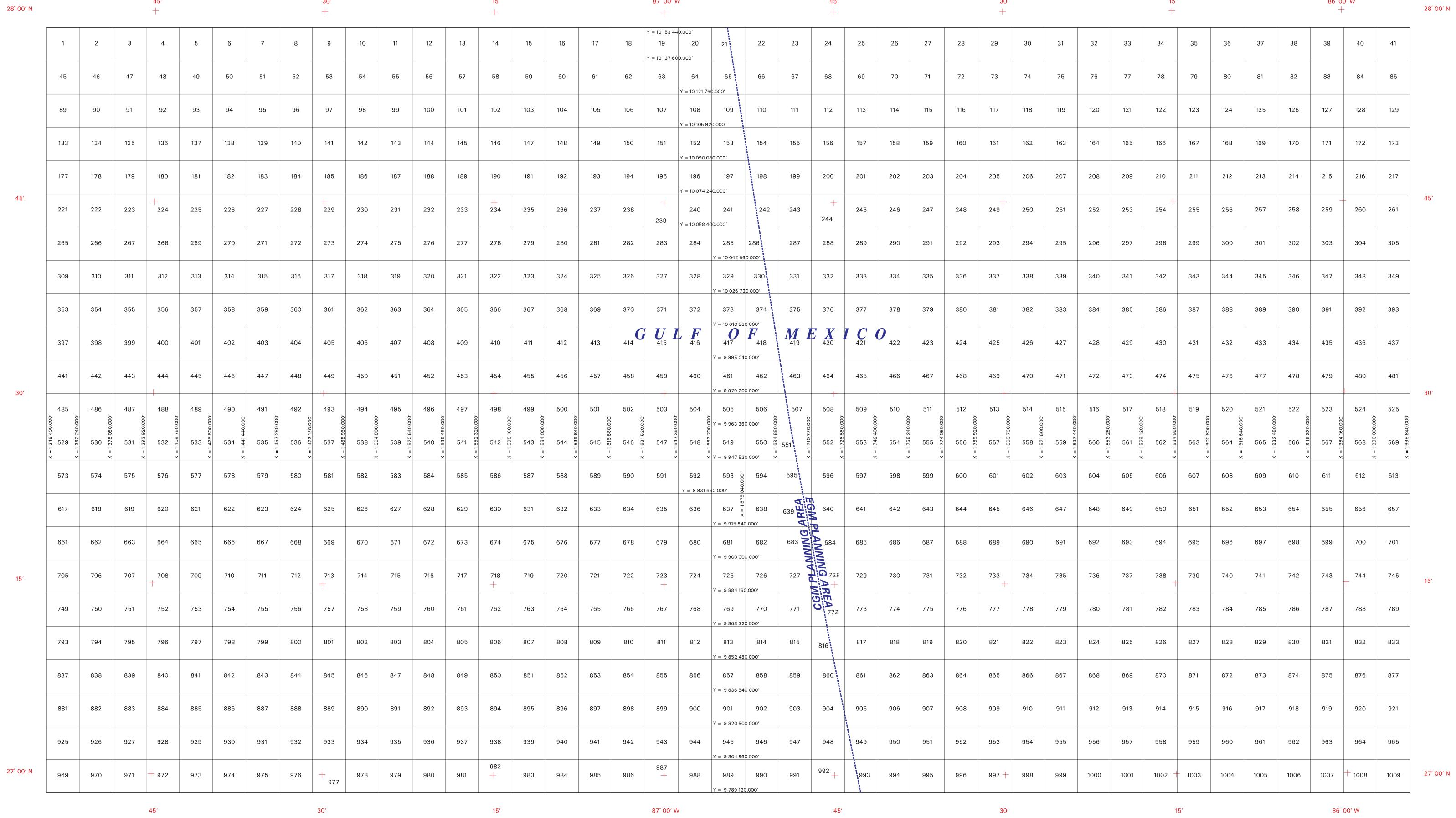
All blocks are based on the Universal Transverse Mercator Grid System, Zone 16, with X origin = 1,640,416.67 feet (500,000 international meters), at  $87^{\circ}$  West Longitude, and Y origin = 0 feet at  $0^{\circ}$  Latitude.
