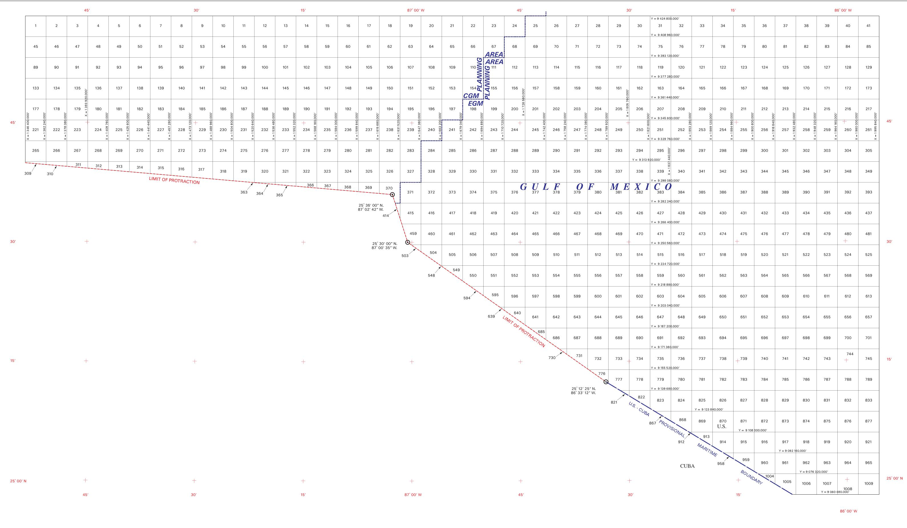
All blocks are based on the Universal Transverse Mercator Grid System, Zone 16, with X origin = 1,640,416.67 feet (500,000 international meters),
