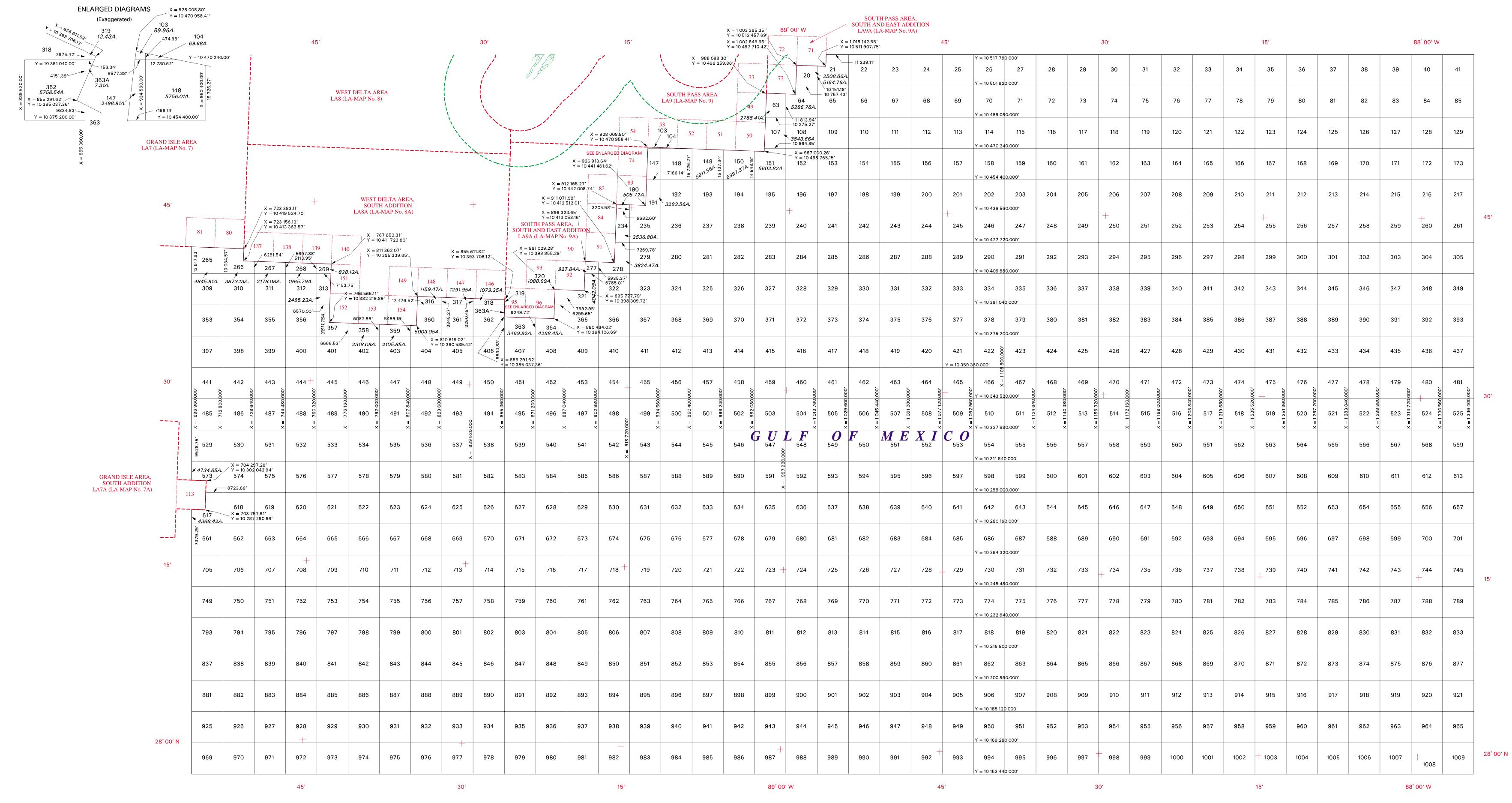
All blocks are based on the Universal Transverse Mercator Grid System, Zone 16, with X origin = 1,640,416.67 feet (500,000 international meters), at  $87^{\circ}$  West Longitude, and Y origin = 0 feet at  $0^{\circ}$  Latitude.
