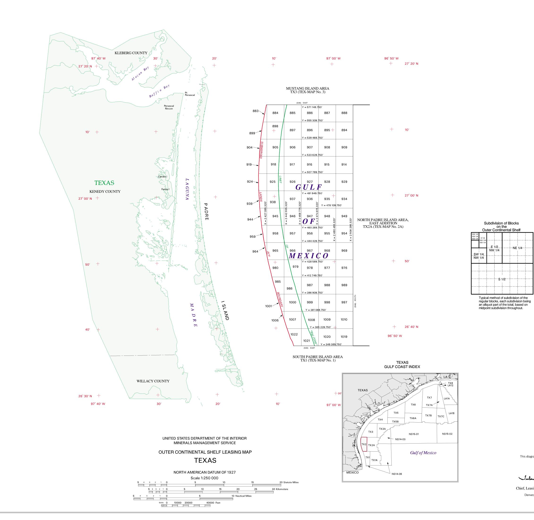
All blocks are based on the Texas (Lambert) Plane Coordinate System, South Zone, with X origin = 2,000,000' at  $98^{\circ}30'$  W and Y origin = 0.00' at  $25^{\circ}40'$  N.
