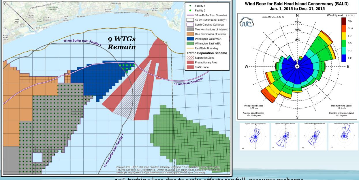
106 turbine loss due to wake effects for full resource recharge
