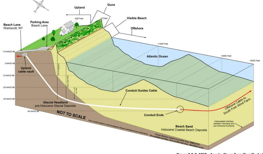
**Figure 3.2-2. SFEC - Sea-to-Shore Transition Illustration** Illustration of sea-to-shore transition at the Beach Lane landing site.
