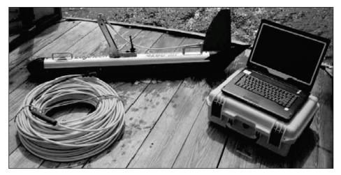
Figure D-21. An Example of a Representative Side-Scan Sonar System. Source: EdgeTech (2011).
