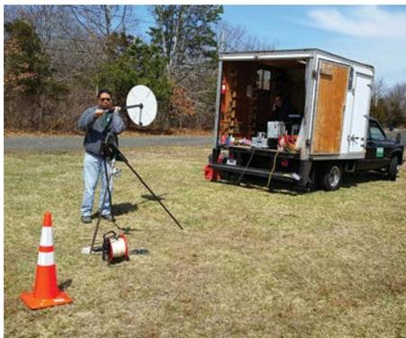
USGS scientist calibrates an electromagnetic induction borehole probe as part of the geophysical data collection at monitoring wells on Shinnecock Nation Tribal Lands. Photo credit: USGS
