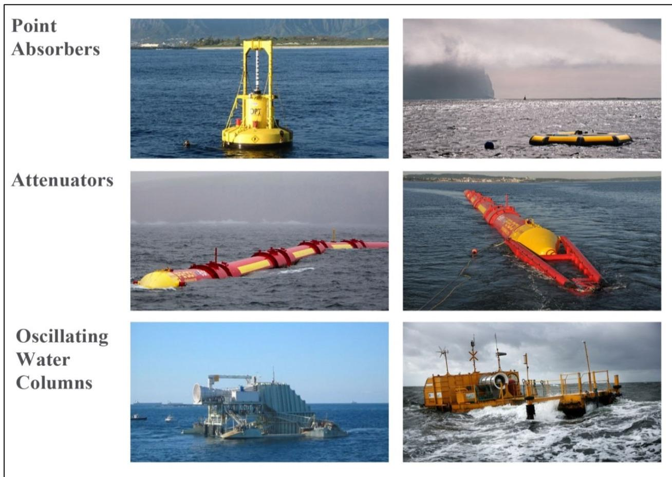
Figure 0-1. Examples of different types of WECs.
