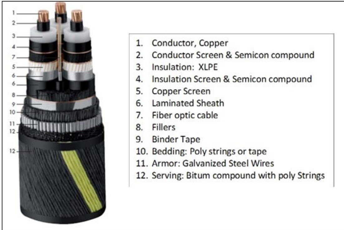
Figure 0-8. Example of medium-voltage subsea cable.
