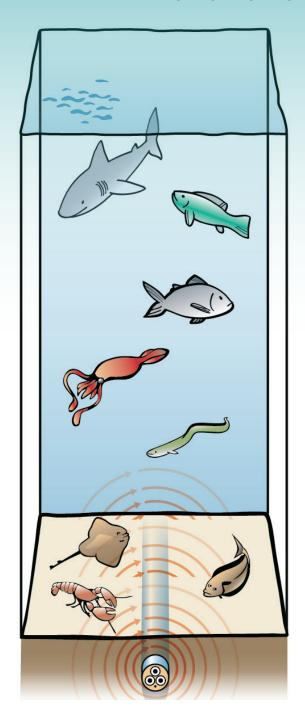
Naturally occurring EMF are present everywhere in the oceans. Undersea cables used for power transfer are known sources of EMF, but telecommunication cables and undersea communication cables also generate alternating current (AC) and direct current (DC) EMF.
