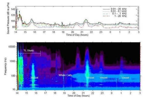
Figure 4. Lower: spectrogram of sound level measurements obtained from a hydrophone recording system. Upper: broadband and selected band level variation with time.
