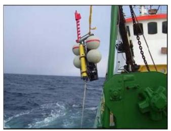
Figure 2. Hydrophone recording system being deployed at sea. The hydrophone system is an autonomous recorder with very high recording resolution. Acoustic data is stored internally on a hard-drive.
