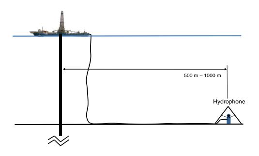
Figure 1. Cabled hydrophone method for real time monitoring of drilling sound energy.
