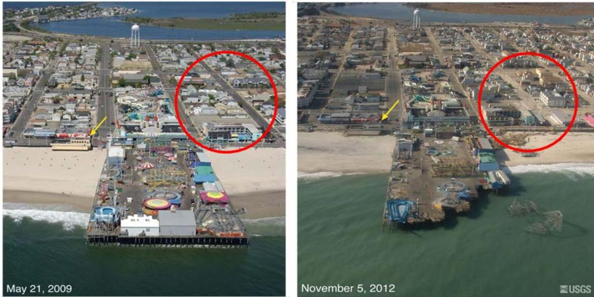
Figure 20. Before and after Hurricane Sandy storm damages (Seaside Heights, New Jersey).
