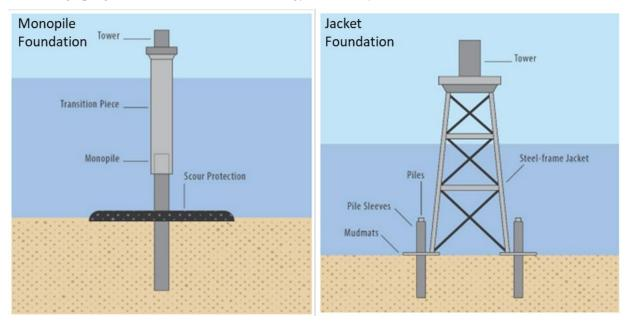
Figure 7. Examples of Monopile and Jacket Foundations
