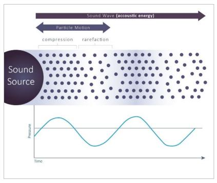
Figure J-1 Basic Mechanics of an Underwater Sound Wave
