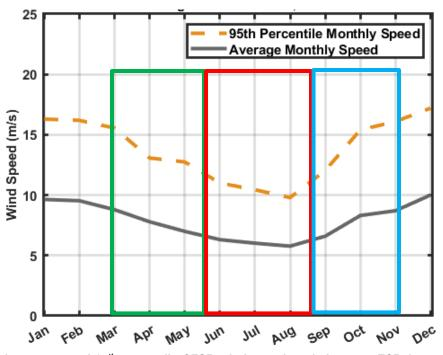
Figure 12. Monthly average and 95<sup>th</sup> percentile CFSR wind speed statistics near ESP 1: monthly average (grey solid) and 95<sup>th</sup> percentile (orange dashed); wind speed reported in m/s. Spring, Summer and Fall seasons are shown by green, red and blue boxes, respectively.
