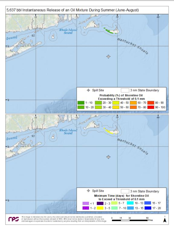
Figure 33. Top Panel—Probability of shoreline oiling above a minimum thickness of 100  $\mu$ m (100 g/m<sup>2</sup> on average over the grid cell) during summer months for an instantaneous discharge from the ESP 1 location. Bottom Panel—Minimum time for shoreline oiling to occur at thicknesses greater than 100 g/m<sup>2</sup>.
