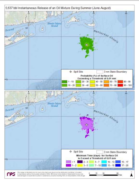
Figure 29. Top Panel–Probability of surface oiling above a minimum thickness of 10  $\mu$ m (10 g/m<sup>2</sup> on average over the grid cell) during summer months for an instantaneous discharge from the ESP 1 location. Bottom Panel–Minimum time for surface oiling to occur at thicknesses greater than 10 g/m<sup>2</sup>.
