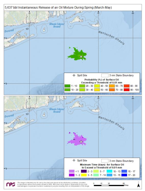
Figure 36. Top Panel—Probability of surface oiling above a minimum thickness of 10  $\mu$ m (10 g/m<sup>2</sup> on average over the grid cell) during spring months for an instantaneous discharge from the ESP 2 location. Bottom Panel—Minimum time for surface oiling to occur at thicknesses greater than 10 g/m<sup>2</sup>.
