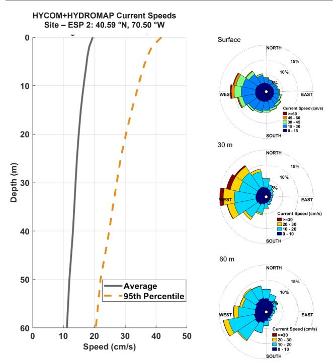
Figure 24. HYCOM average (solid grey) and 95<sup>th</sup> percentile (dashed orange) of horizontal current speed (cm/s) dataset from 2001-2010, variation with depth near ESP 2; and the current roses at surface, 30 m, and 60 m water depths. The roses show the direction that current is flowing towards.
