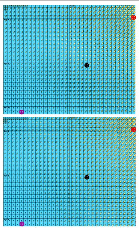
Figure 16. Illustration showing flood (upper panel) and ebb current pattern (lower panel) near ESP 1, ESP 2, and OOI Pioneer Inshore Surface Mooring showed by red, black, and purple marks, respectively.
