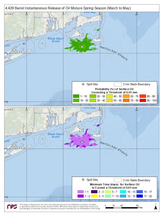
Figure A-17. Detail View. Top Panel—Probability of surface oiling above a minimum thickness of 10  $\mu$ m (10 g/m<sup>2</sup> on average over the grid cell) during spring months for an instantaneous discharge from the potential booster station. Bottom Panel—Minimum time for surface oiling to occur at thicknesses greater than 10 g/m<sup>2</sup>.
