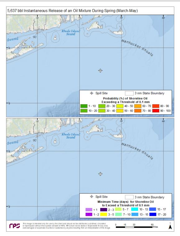
Figure 40. Top Panel—Probability of shoreline oiling above a minimum thickness of 100  $\mu$ m (100 g/m<sup>2</sup> on average over the grid cell) during spring months for an instantaneous discharge from the ESP 2 location. Bottom Panel—Minimum time for shoreline oiling to occur at thicknesses greater than 100 g/m<sup>2</sup>.
