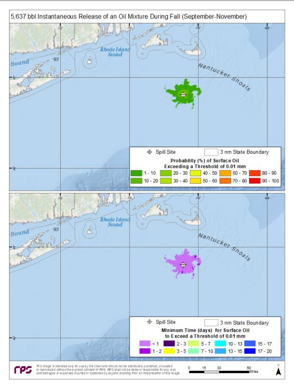
Figure 30. Top Panel—Probability of surface oiling above a minimum thickness of 10  $\mu$ m (10 g/m<sup>2</sup> on average over the grid cell) during fall months for an instantaneous discharge from the ESP 1 location. Bottom Panel—Minimum time for surface oiling to occur at thicknesses greater than 10 g/m<sup>2</sup>.
