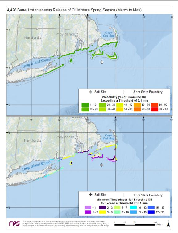
Figure A-24. Top Panel—Probability of shoreline oiling above a minimum thickness of 100  $\mu$ m (100 g/m<sup>2</sup> on average over the grid cell) during spring months for an instantaneous discharge from the potential booster station. Bottom Panel—Minimum time for shoreline oiling to occur at thicknesses greater than 100 g/m<sup>2</sup>.
