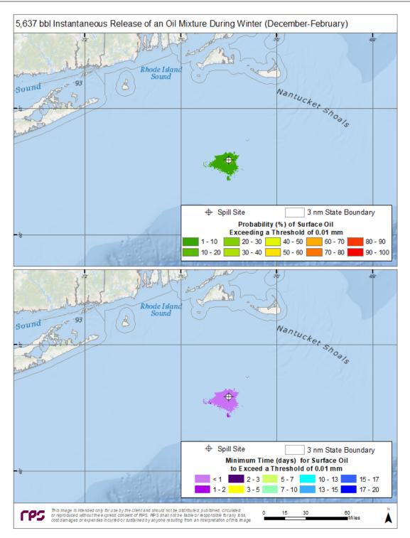
Figure 39. Top Panel—Probability of surface oiling above a minimum thickness of 10  $\mu$ m (10 g/m<sup>2</sup> on average over the grid cell) during winter months for an instantaneous discharge from the ESP 2 location. Bottom Panel—Minimum time for surface oiling to occur at thicknesses greater than 10 g/m<sup>2</sup>.
