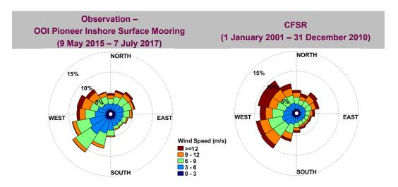
Figure 7. Comparison between wind measurement and CFSR at OOI Pioneer Inshore Surface Mooring.
