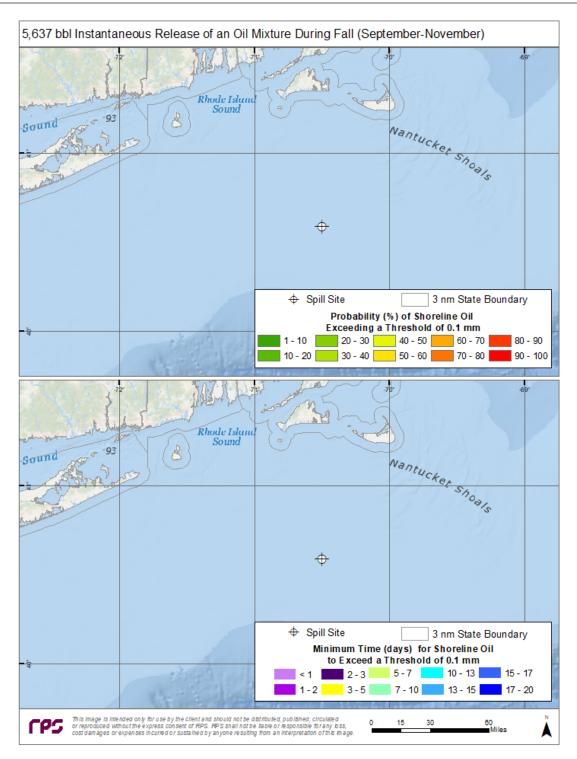
Figure 42. Top Panel—Probability of shoreline oiling above a minimum thickness of 100  $\mu$ m (100 g/m<sup>2</sup> on average over the grid cell) during fall months for an instantaneous discharge from the ESP 2 location. Bottom Panel—Minimum time for shoreline oiling to occur at thicknesses greater than 100 g/m<sup>2</sup>.
