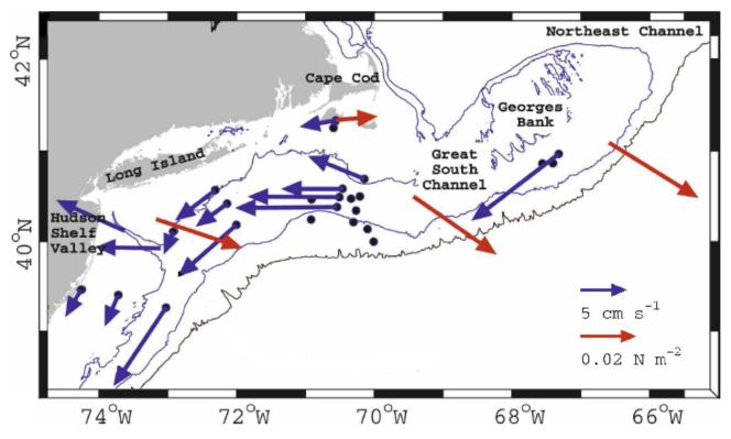
Figure 3. Map of the MAB showing mean depth-averaged current vectors in blue, and mean wind stress vectors in red based on observations (modified from Lentz 2008).
