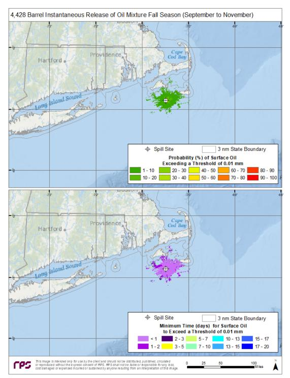
Figure A-20. Top Panel—Probability of surface oiling above a minimum thickness of 10  $\mu$ m (10 g/m<sup>2</sup> on average over the grid cell) during fall months for an instantaneous discharge from the potential booster station. Bottom Panel—Minimum time for surface oiling to occur at thicknesses greater than 10 g/m<sup>2</sup>.
