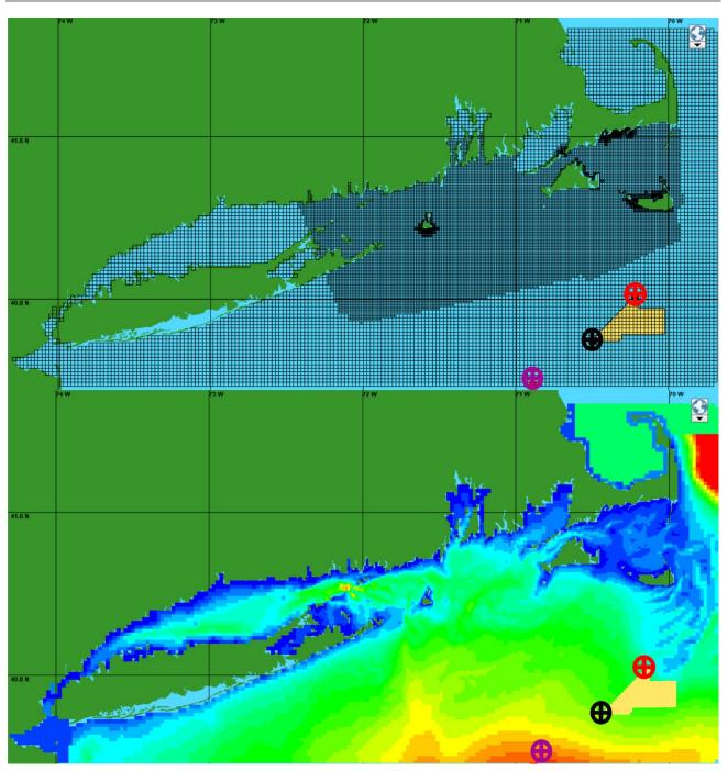
Figure 14. Illustration of the HYDROMAP model grid (upper panel) and bathymetry (relative to Mean Sea Level) (lower panel) for entire tidal domain. Red mark shows ESP 1, black mark shows ESP 2, and purple mark shows OOI Pioneer Inshore Surface Mooring. The yellow area between ESP 1 and ESP 2 is Lease Area OCS-A 0522.
