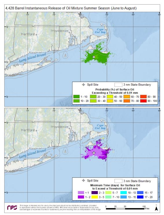
Figure A-18. Top Panel—Probability of surface oiling above a minimum thickness of 10  $\mu$ m (10 g/m<sup>2</sup> on average over the grid cell) during summer months for an instantaneous discharge from the potential booster station. Bottom Panel—Minimum time for surface oiling to occur at thicknesses greater than 10 g/m<sup>2</sup>.
