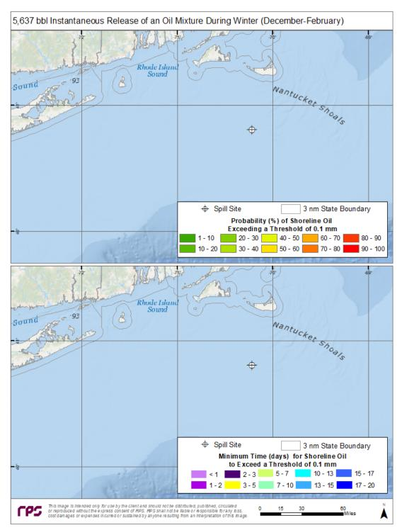
Figure 35. Top Panel—Probability of shoreline oiling above a minimum thickness of 100  $\mu$ m (100 g/m<sup>2</sup> on average over the grid cell) during winter months for an instantaneous discharge from the ESP 1 location. Bottom Panel—Minimum time for shoreline oiling to occur at thicknesses greater than 100 g/m<sup>2</sup>.
