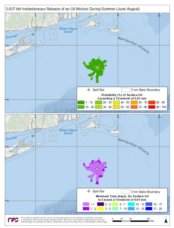
Figure 37. Top Panel—Probability of surface oiling above a minimum thickness of 10  $\mu$ m (10 g/m<sup>2</sup> on average over the grid cell) during summer months for an instantaneous discharge from the ESP 2 location. Bottom Panel—Minimum time for surface oiling to occur at thicknesses greater than 10 g/m<sup>2</sup>.
