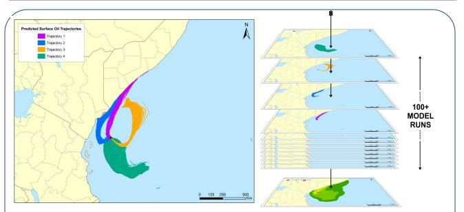
Examples of four individual spill trajectories predicted by OILMAP/SIMAP for a particular spill scenario. The frequency of contact with given locations is used to calculate the probability of impacts during a spill. Essentially, all 100+ model runs are overlain (shown as the stacked runs on the right) and the number of times that a trajectory reaches a given location is used to calculate the probability for that location.
