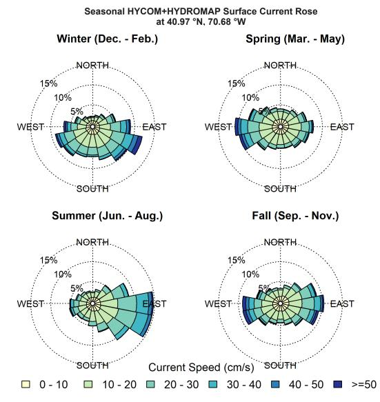
Figure A-13. Seasonal HYCOM+HYDROMAP current roses in the vicinity of the booster station. Current speeds in cm/s, using oceanographic convention (direction currents are heading towards).
