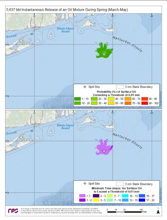
Figure 28. Top Panel—Probability of surface oiling above a minimum thickness of 10  $\mu$ m (10 g/m<sup>2</sup> on average over the grid cell) during spring months for an instantaneous discharge from the ESP 1 location. Bottom Panel—Minimum time for surface oiling to occur at thicknesses greater than 10 g/m<sup>2</sup>.
