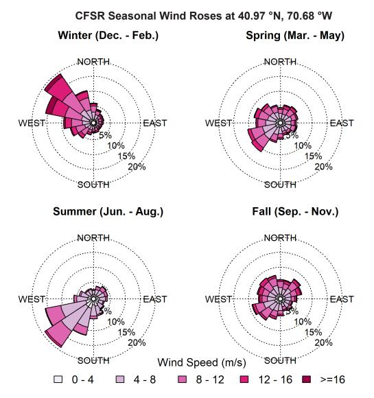
Figure A-7. Seasonal CFSR wind roses in the vicinity of the booster station. Wind speeds in m/s, using meteorological convention (i.e., direction wind is coming from).
