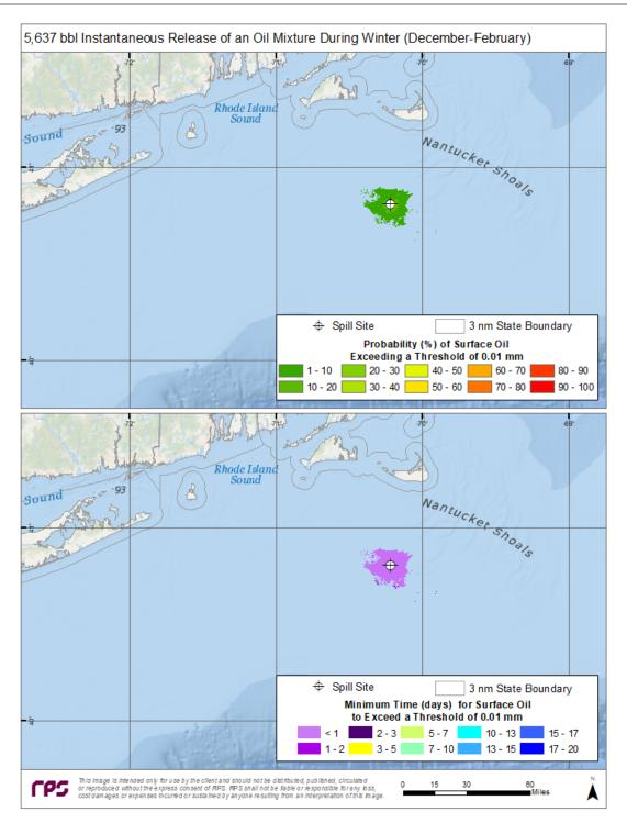
Figure 31. Top Panel—Probability of surface oiling above a minimum thickness of 10  $\mu$ m (10 g/m<sup>2</sup> on average over the grid cell) during winter months for an instantaneous discharge from the ESP 1 location. Bottom Panel—Minimum time for surface oiling to occur at thicknesses greater than 10 g/m<sup>2</sup>.
