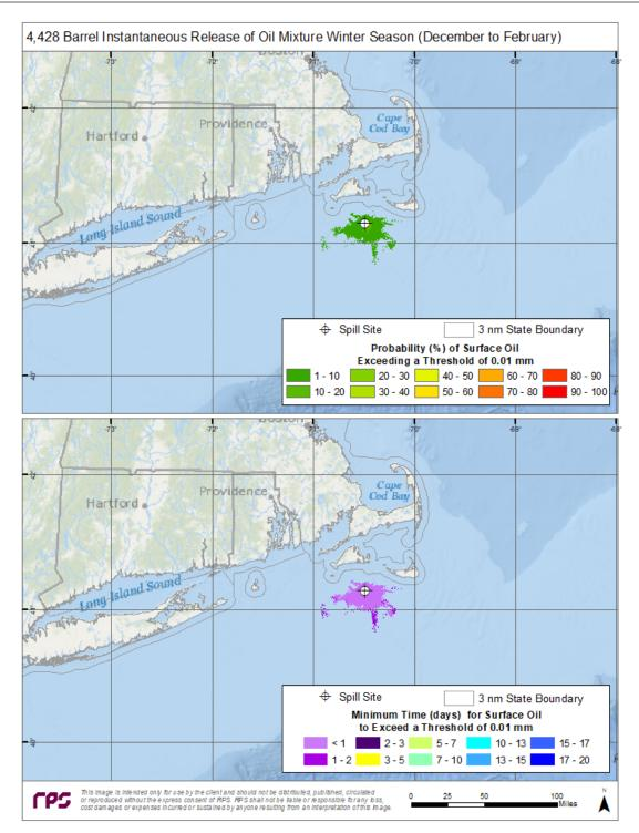
Figure A-22. Top Panel—Probability of surface oiling above a minimum thickness of 10  $\mu$ m (10 g/m<sup>2</sup> on average over the grid cell) during winter months for an instantaneous discharge from the potential booster station. Bottom Panel—Minimum time for surface oiling to occur at thicknesses greater than 10 g/m<sup>2</sup>.
