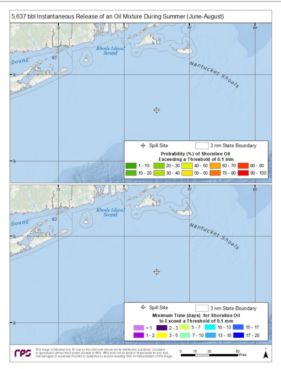
Figure 41. Top Panel—Probability of shoreline oiling above a minimum thickness of 100  $\mu$ m (100 g/m<sup>2</sup> on average over the grid cell) during summer months for an instantaneous discharge from the ESP 2 location. Bottom Panel—Minimum time for shoreline oiling to occur at thicknesses greater than 100 g/m<sup>2</sup>.
