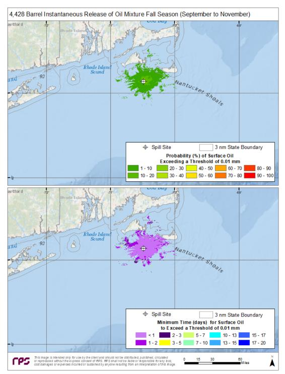
Figure A-21. Detail View. Top Panel—Probability of surface oiling above a minimum thickness of 10  $\mu$ m (10 g/m<sup>2</sup> on average over the grid cell) during fall months for an instantaneous discharge from the potential booster station. Bottom Panel—Minimum time for surface oiling to occur at thicknesses greater than 10 g/m<sup>2</sup>.
