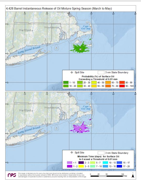
Figure A-16. Top Panel—Probability of surface oiling above a minimum thickness of 10  $\mu$ m (10 g/m<sup>2</sup> on average over the grid cell) during spring months for an instantaneous discharge from the potential booster station. Bottom Panel—Minimum time for surface oiling to occur at thicknesses greater than 10 g/m<sup>2</sup>.
