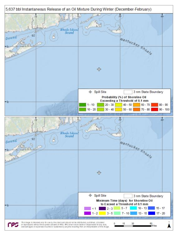
Figure 43. Top Panel—Probability of shoreline oiling above a minimum thickness of 100  $\mu$ m (100 g/m<sup>2</sup> on average over the grid cell) during winter months for an instantaneous discharge from the ESP 2 location. Bottom Panel—Minimum time for shoreline oiling to occur at thicknesses greater than 100 g/m<sup>2</sup>.
