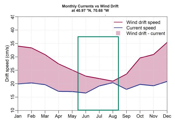
Figure A-14. Surface drift forcing comparison statistics in the vicinity of the booster station: monthly-averaged CSFR wind drift compared with HYCOM+HYDROMAP current speed. Wind drift is calculated as 3.5% of the wind speed. Periods with predominant wind transport are shaded pink. The green box highlights summer.
