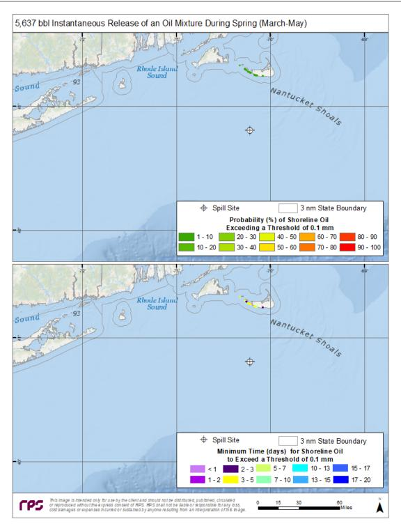
Figure 32. Top Panel—Probability of shoreline oiling above a minimum thickness of 100  $\mu$ m (100 g/m<sup>2</sup> on average over the grid cell) during spring months for an instantaneous discharge from the ESP 1 location. Bottom Panel—Minimum time for shoreline oiling to occur at thicknesses greater than 100 g/m<sup>2</sup>.
