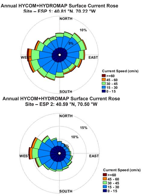
Figure 19. Annual HYCOM + HYDROMAP roses near ESP 1 (upper panel) and ESP 2 (lower panel) for 2001-2010. Current speeds in cm/s, using oceanographic convention (i.e., direction current is going to).
