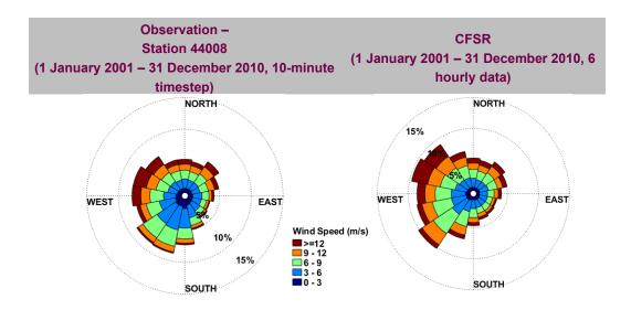
Figure 9. Comparison between wind measurement and CFSR at Station 44008.
