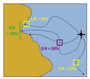
Figure A-15. Example illustration of the difference between surface and shoreline oiling probabilities. Surface probabilities in yellow and purple, shoreline probabilities in green.
