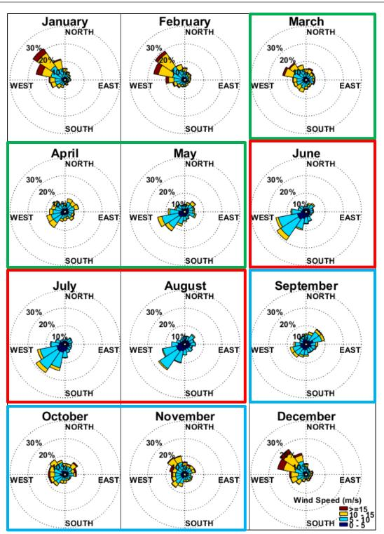
Figure 13. Monthly CFSR wind roses near ESP 1. Wind speeds in m/s, using meteorological convention (i.e., direction wind is coming from). Spring, Summer and Fall seasons are shown by green, red, and blue boxes, respectively.
