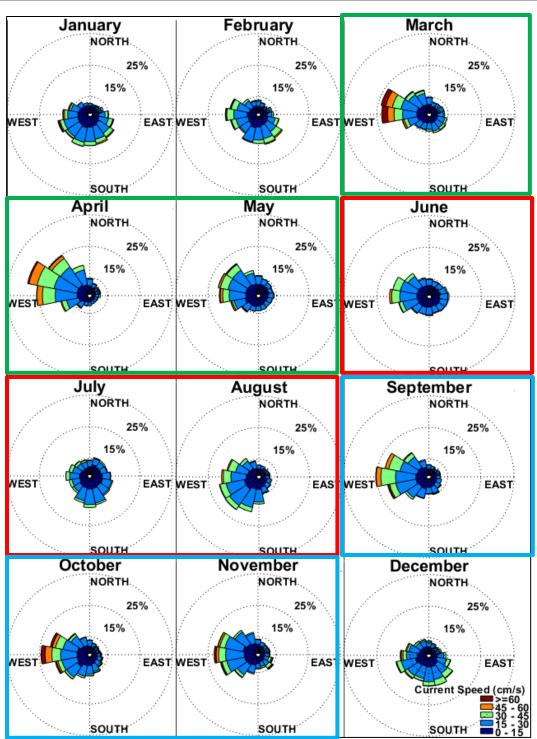
Figure 22. Monthly HYCOM + HYDROMAP surface current roses near ESP 2 for 2001-2010; following oceanographic convention (currents heading to), current speeds in cm/s Spring, Summer and Fall seasons are shown by green, red and blue boxes, respectively.
