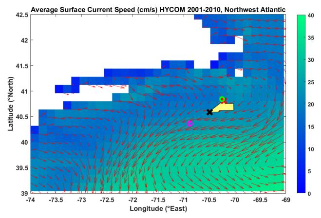
Figure 18. HYCOM surface current speed averaged over 2001-2010, Northwest Atlantic. Red and black "X"s show spill sites ESP 1 and ESP 2, respectively. The observation site of OOI Pioneer Inshore Surface Mooring is shown by the purple circle. The yellow area between ESP 1 and ESP 2 is Lease Area OCS-A 0522.
