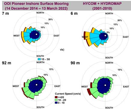
Figure 17. Comparison between current measurement and HYCOM + HYDROMAP output at OOI Pioneer Inshore Surface Mooring.
