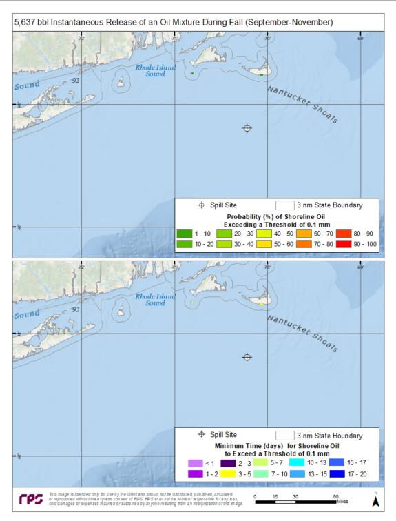
Figure 34. Top Panel—Probability of shoreline oiling above a minimum thickness of 100  $\mu$ m (100 g/m<sup>2</sup> on average over the grid cell) during fall months for an instantaneous discharge from the ESP 1 location. Bottom Panel—Minimum time for shoreline oiling to occur at thicknesses greater than 100 g/m<sup>2</sup>.
