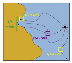
Figure 27. Example illustration of the difference between surface and shoreline oiling probabilities. Surface probabilities in yellow and purple, shoreline probabilities in green.
