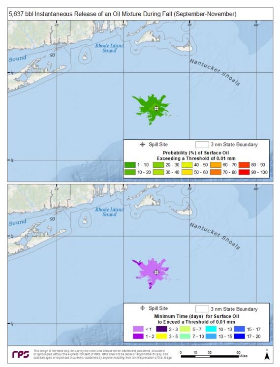
Figure 38. Top Panel—Probability of surface oiling above a minimum thickness of 10  $\mu$ m (10 g/m<sup>2</sup> on average over the grid cell) during fall months for an instantaneous discharge from the ESP 2 location. Bottom Panel—Minimum time for surface oiling to occur at thicknesses greater than 10 g/m<sup>2</sup>.
