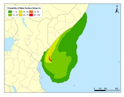
Probability of surface oil exceeding a given threshold for the example scenario. This figure overlays 100+ individual model runs to calculate the percentage of runs that caused oiling above the threshold in a given area. This figure does not depict the areal extent of a single model run/spill.
