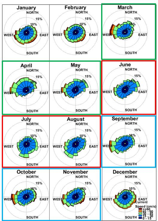
Figure 21. Monthly HYCOM + HYDROMAP surface current roses near ESP 1 for 2001-2010; following oceanographic convention (currents heading to), current speeds in cm/s. Spring, Summer and Fall seasons are shown by green, red and blue boxes, respectively.
