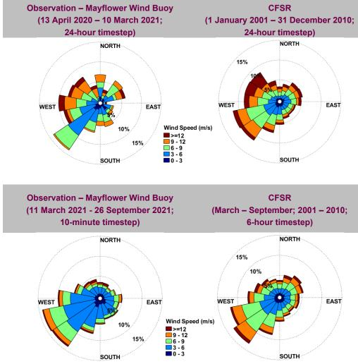
Figure 8. Comparison between wind measurement and CFSR at Mayflower Wind Buoy.
