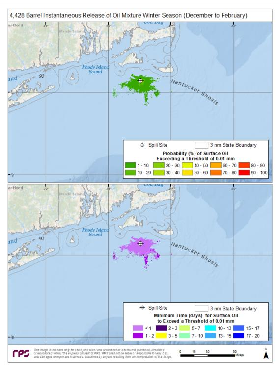
Figure A-23. Detail View. Top Panel—Probability of surface oiling above a minimum thickness of 10  $\mu$ m (10 g/m<sup>2</sup> on average over the grid cell) during winter months for an instantaneous discharge from the potential booster station. Bottom Panel—Minimum time for surface oiling to occur at thicknesses greater than 10 g/m<sup>2</sup>.
