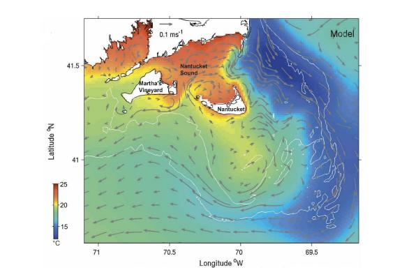
the tidal residual anticyclonic flow encircling the Nantucket Shoals and prevails the wind-driven flow (Figure 4; Wilkin 2006).
