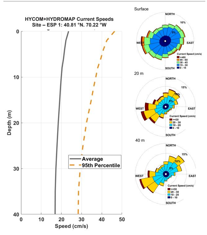
Figure 23. HYCOM average (solid grey) and 95<sup>th</sup> percentile (dashed orange) of horizontal current speed (cm/s) dataset from 2001-2010, variation with depth near ESP 1; and the current roses at surface, 20 m, and 40 m water depths. The roses show the direction that current is flowing towards.
