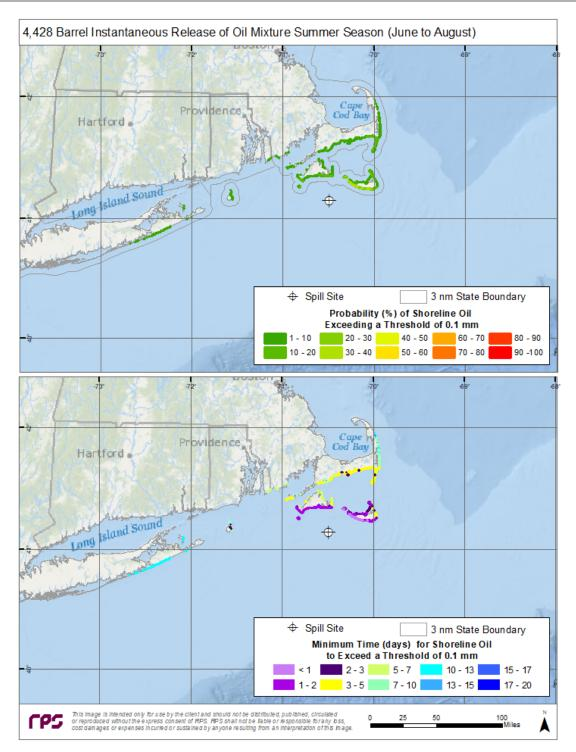
Figure A-25. Top Panel—Probability of shoreline oiling above a minimum thickness of 100  $\mu$ m (100 g/m<sup>2</sup> on average over the grid cell) during summer months for an instantaneous discharge from the potential booster station. Bottom Panel—Minimum time for shoreline oiling to occur at thicknesses greater than 100 g/m<sup>2</sup>.
