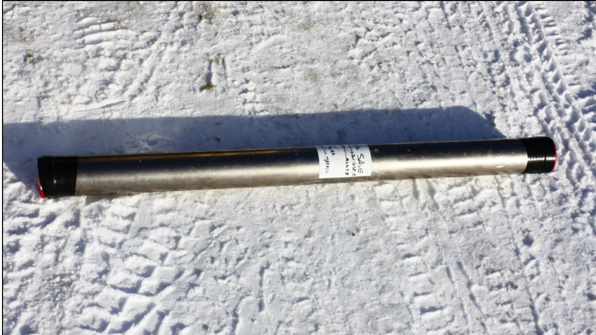
Figure 9. Dedicated core before opening steel core barrel. Core length is 1 m.
