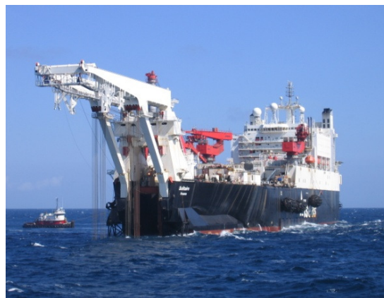
Figure IV-3. S Lay Pipelaying Vessel Allseas' Soltaire
