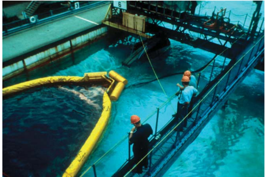
OHMSETT facility test of containment boom and skimmer used to control and recover oil in open waters.
