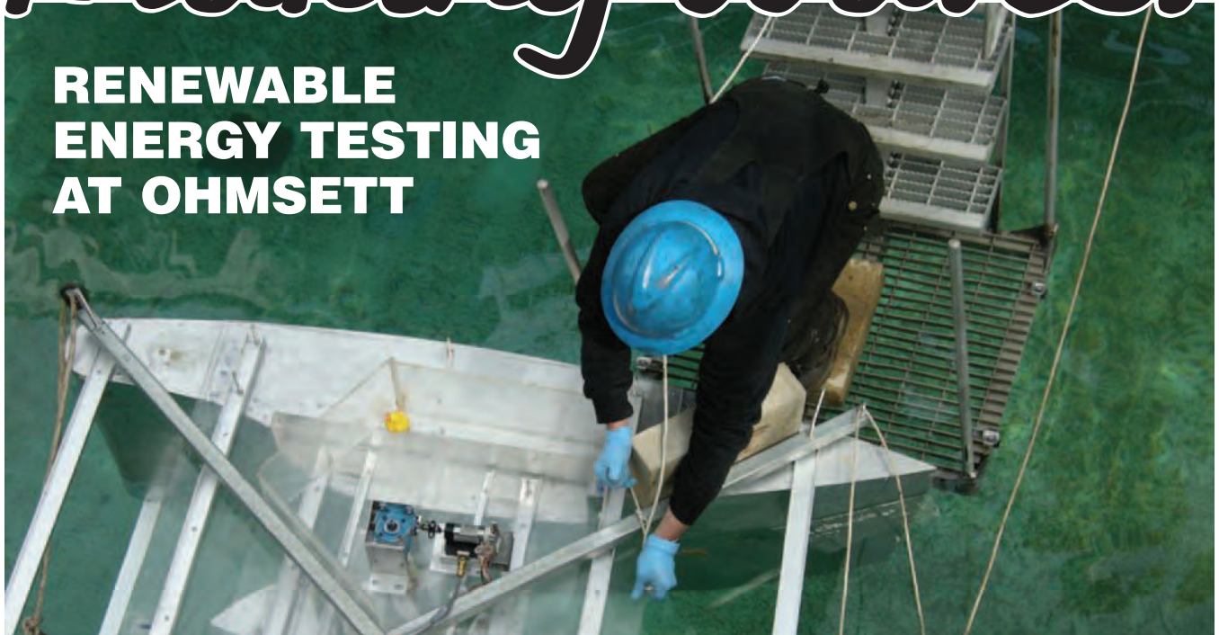
Preparing UNAM's Model 1 hydrodynamic generator for testing in the Ohmsett test tank.
