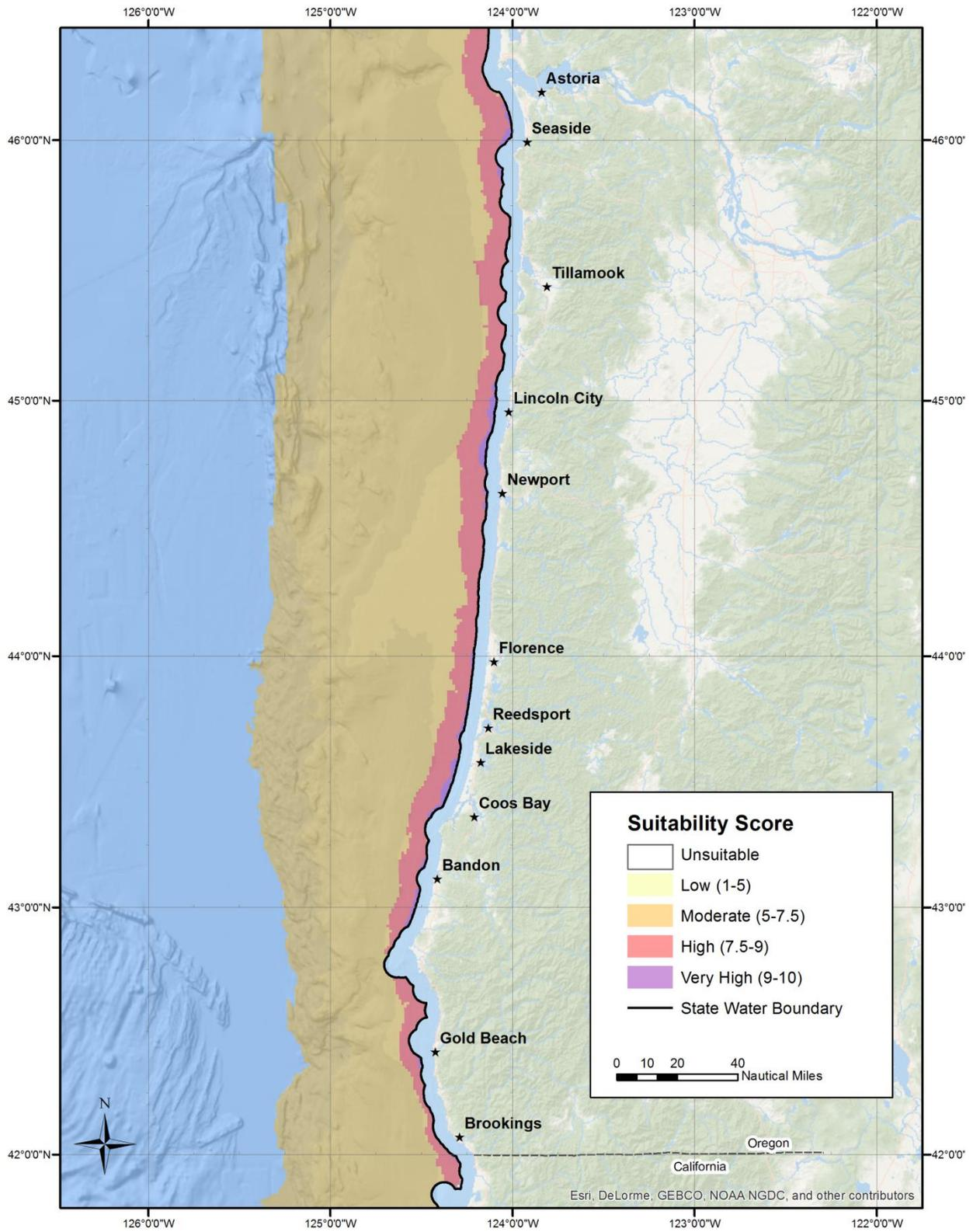
**Figure 7. Site suitability for mid-depth wave energy converter devices.**
