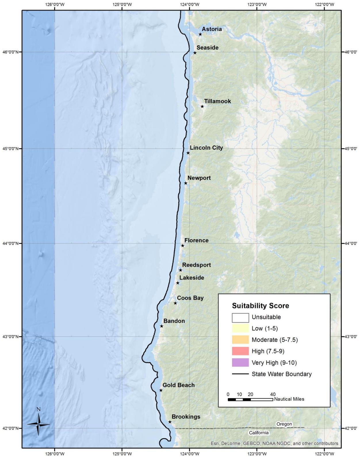
Figure 6. Site suitability for nearshore wave energy converter devices.
