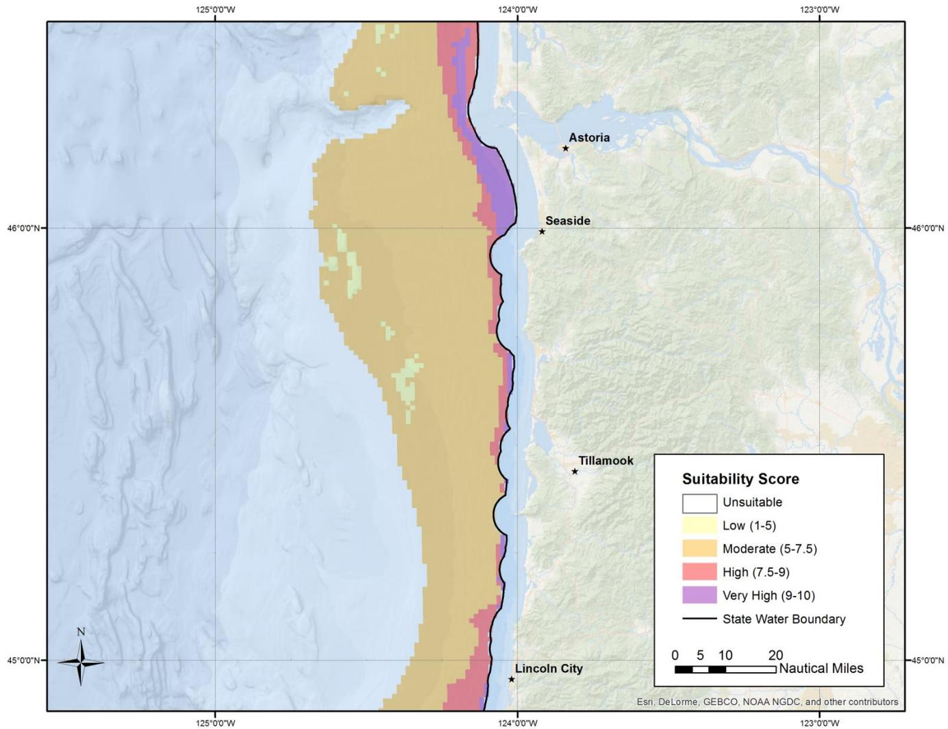
**Figure I.13. Site suitability for jacket/tripod wind energy devices along the northern Oregon Coast.**
