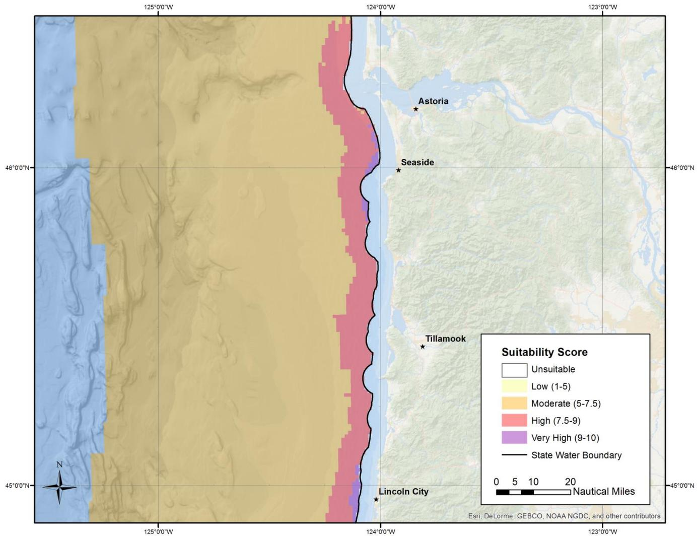
**Figure I.4. Site suitability for mid-depth wave energy converter devices along the northern Oregon Coast.**
