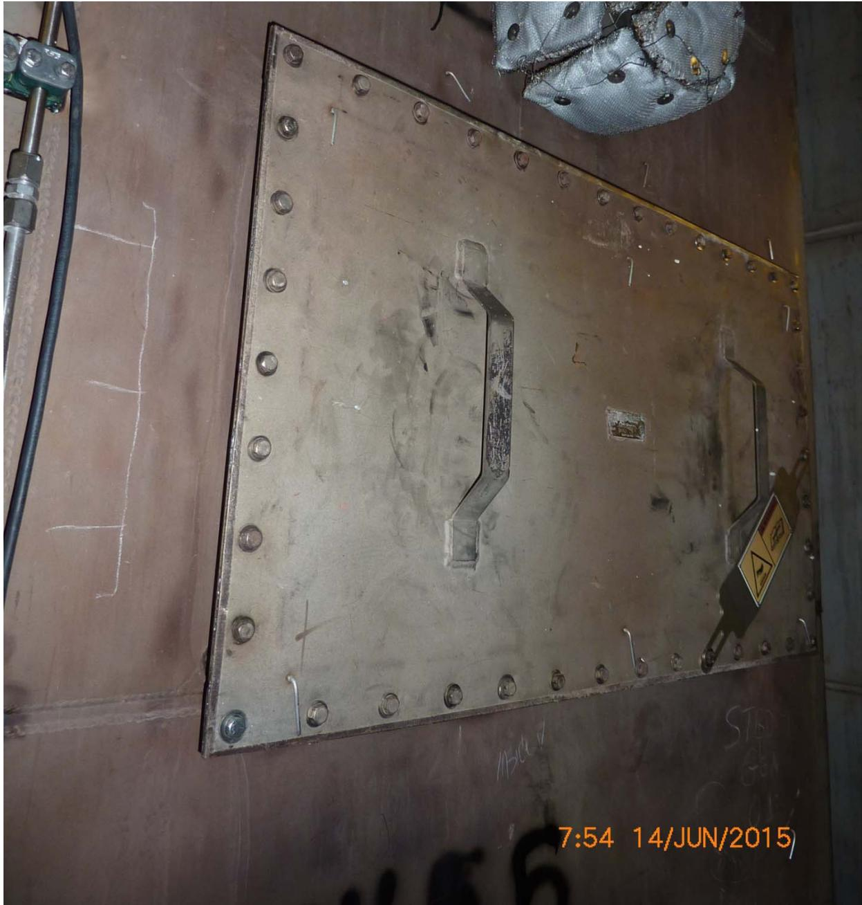
Aiviq 4 – Generator Engine No. 5 – Catalyzed diesel particulate filter housing and urea entry port
