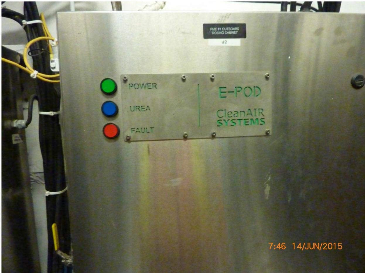
Aiviq 15 – Main Engine No. 2 – SCR urea control panel
