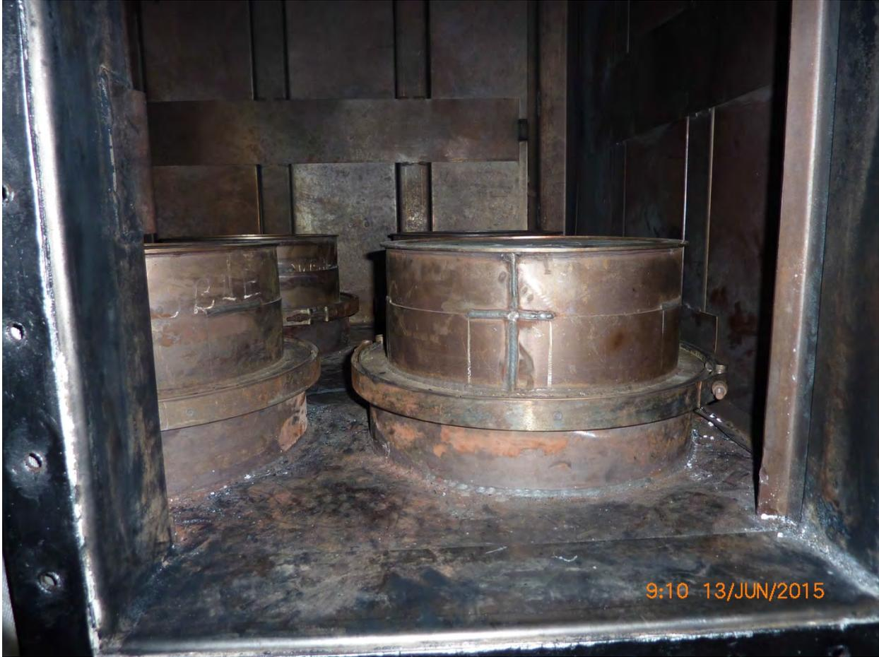
Noble Discoverer 23 – Main Generator Engine No. 1-- Catalyzed diesel particulate filters in housing
