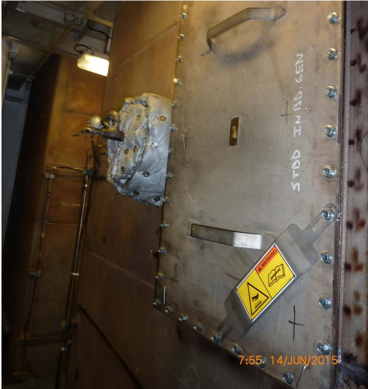
Aiviq 6 – Main Engine No. 2 – Diesel oxidation catalyst housing and urea entry port
