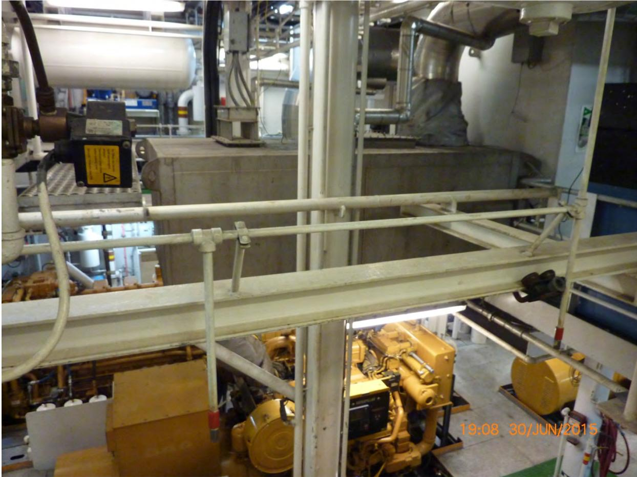
Nanuq 4 – Aft Generator Engine -- Catalyzed Diesel Particulate Filter Housing
