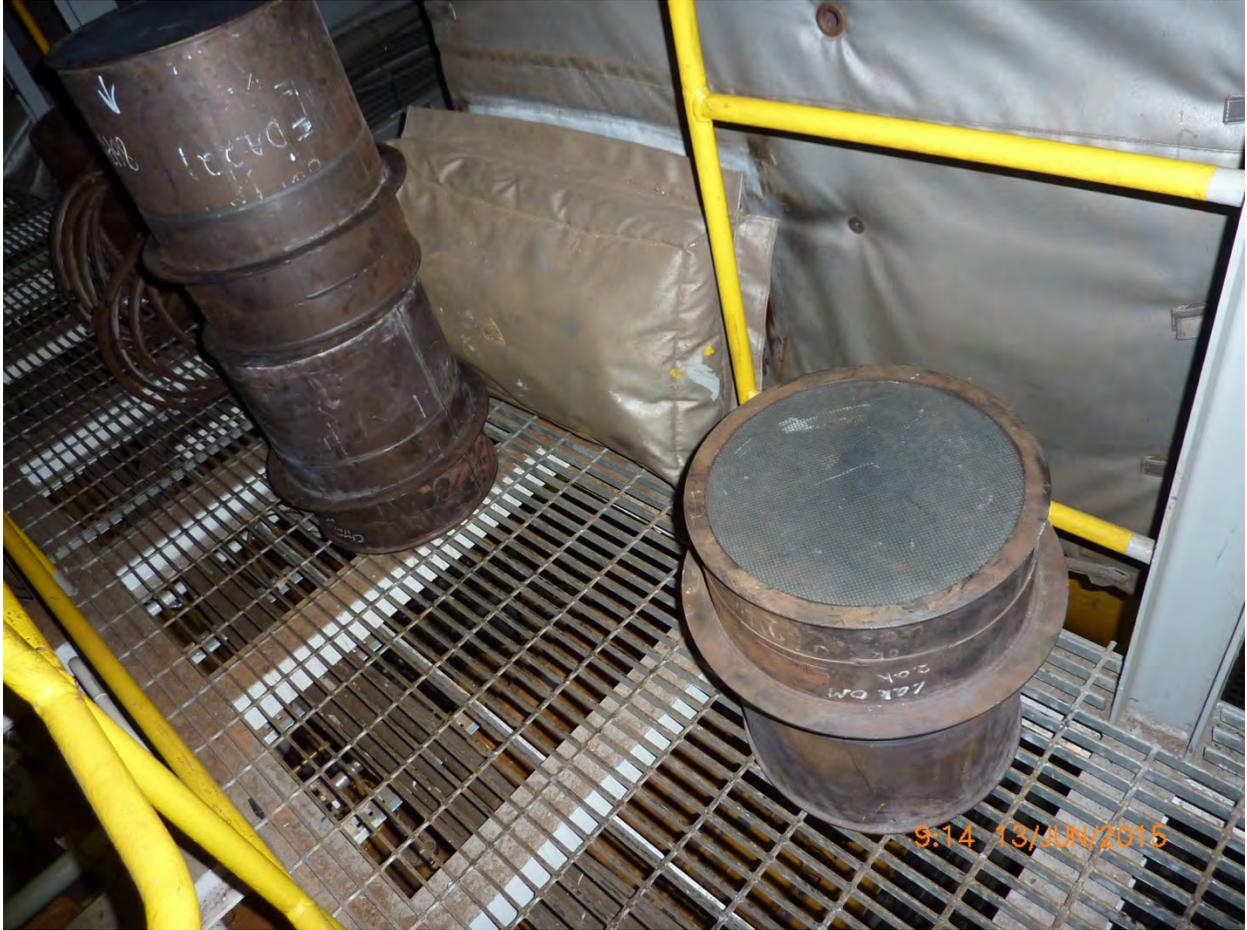
Noble Discoverer 21 – Main Generator Engine No. 3-- Catalyzed diesel particulate filter housing with filters
