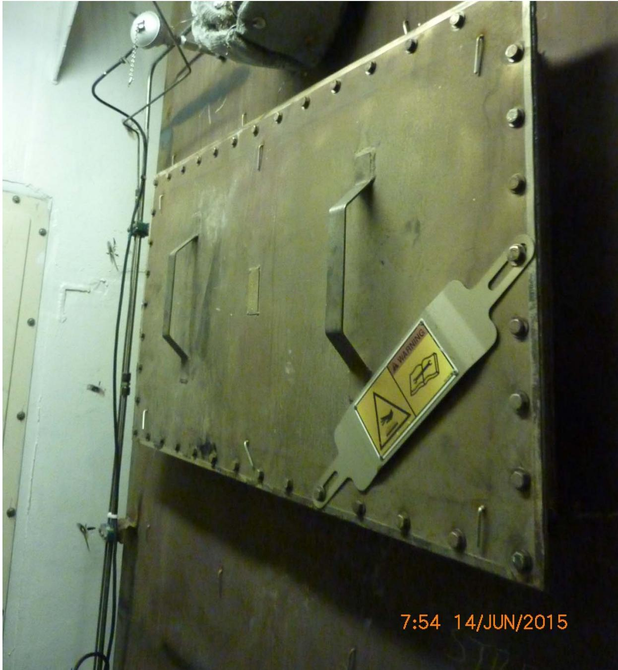
Aiviq 5 – Main Engine No. 1 – Diesel oxidation catalyst housing and urea entry port
