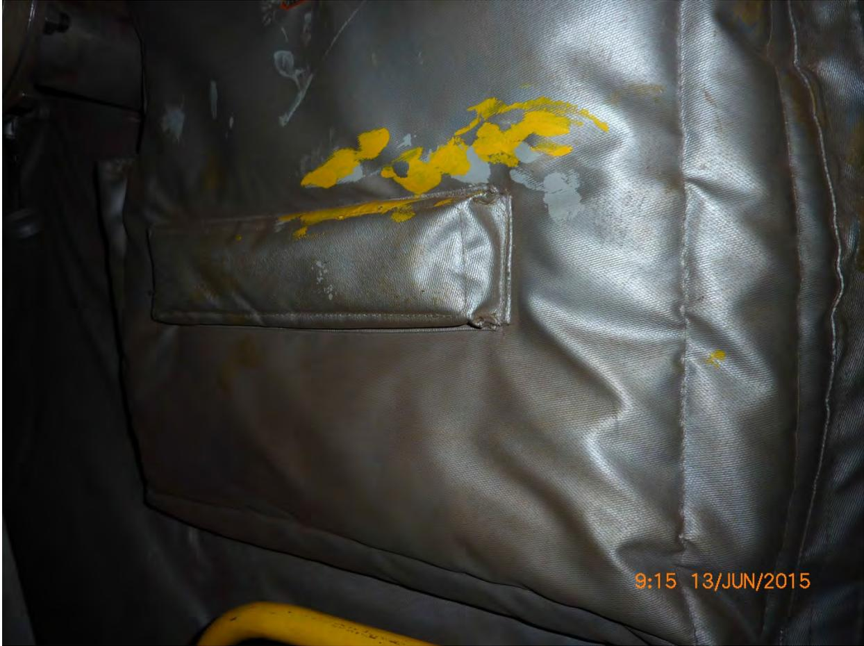
Noble Discoverer 20 – Main Generator Engine No. 4 -- Catalyzed diesel particulate filter housing
