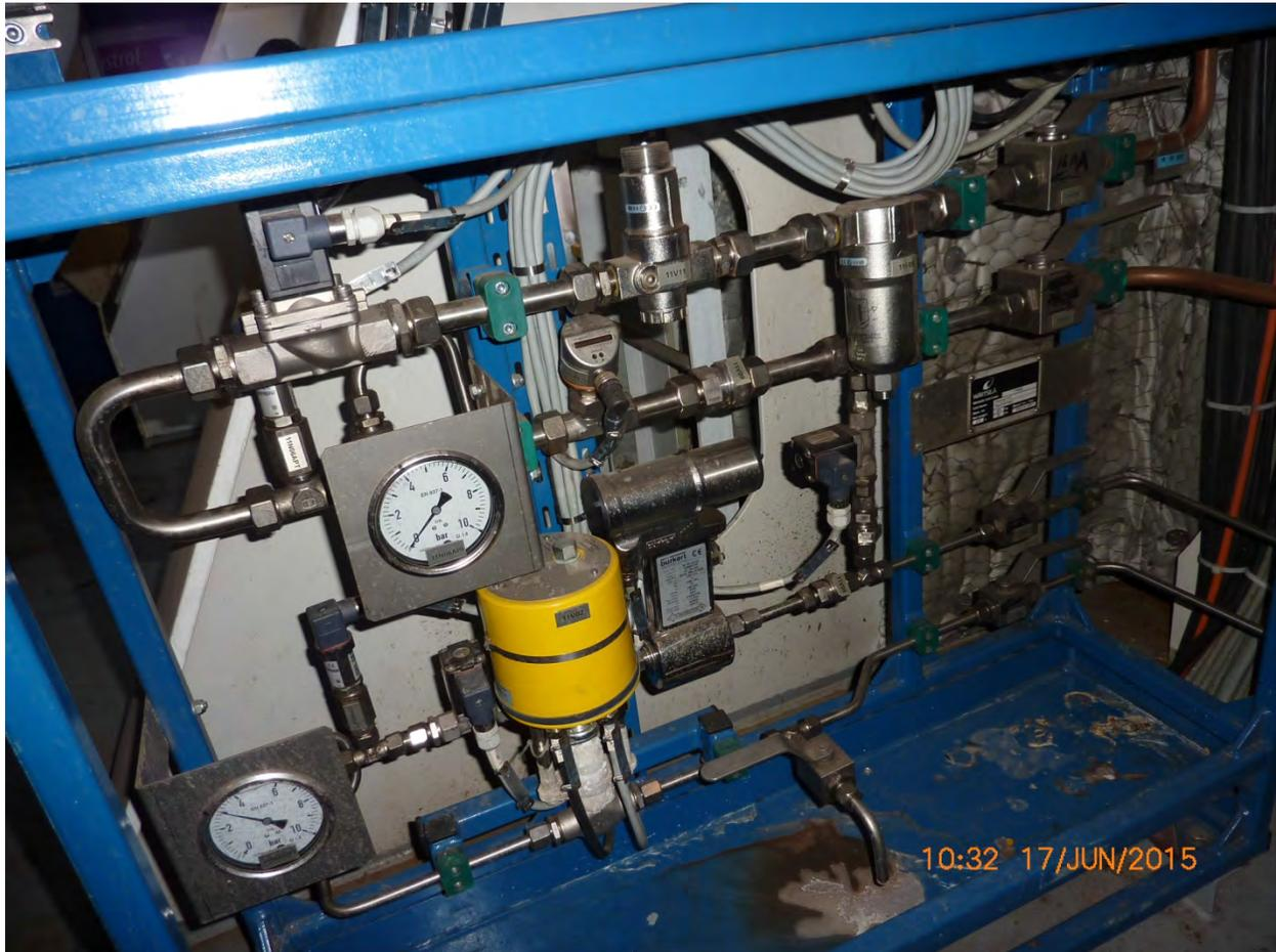
Nordica 16 – Main Engine No. 4 – SCR control valves
