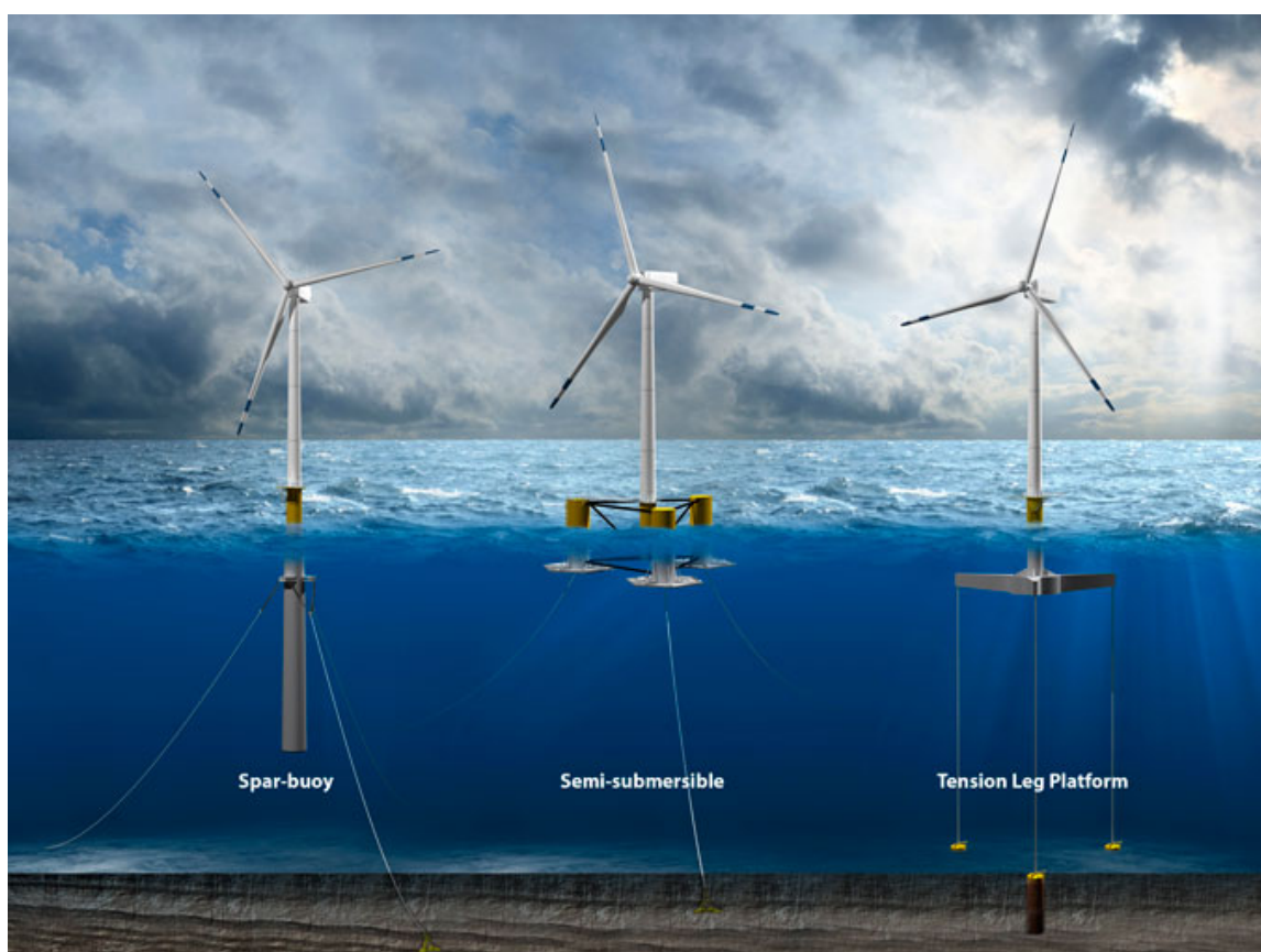
Figure 1-2. Illustration of types of offshore wind turbine platforms
