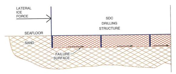
(c) TIP - TO - TIP FAILURE MODE
