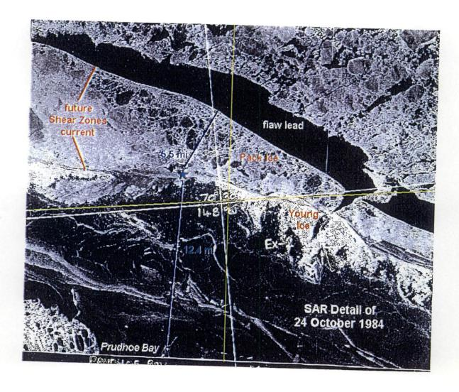
Figure 3: Early Ice Conditions Showing Fast Ice Reaching the Location (Oct 24, 1984).
