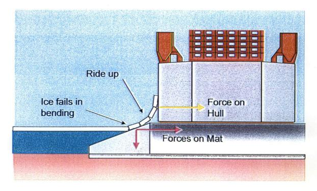
Figure 5: Bending Failure with Ride Up
