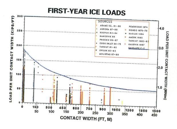
Figure 8: Ice Load Criteria from the Canmar Full Scale Data Base
