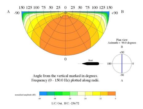
Source Directivity Plot - azimuth : 90.0 degrees - array SeaScan\_2x880\_3M
