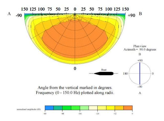
Source Directivity Plot - azimuth : 90.0 degrees - array SeaScan\_USW\_440\_2m
