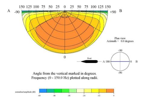
Source Directivity Plot - azimuth : 0.0 degrees - array SeaScan\_USW\_4x220\_2m
