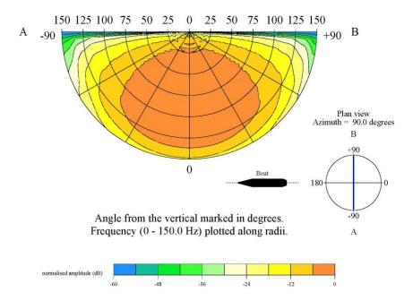
Source Directivity Plot - azimuth : 90.0 degrees - array SeaScan\_USW\_4x220\_2m
