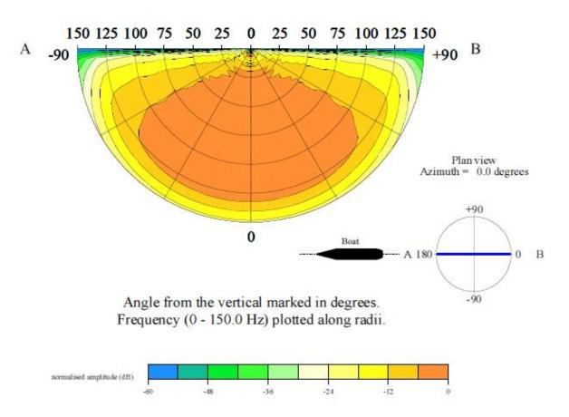
Source Directivity Plot - azimuth : 0.0 degrees - array SeaScan\_USW\_440\_2m
