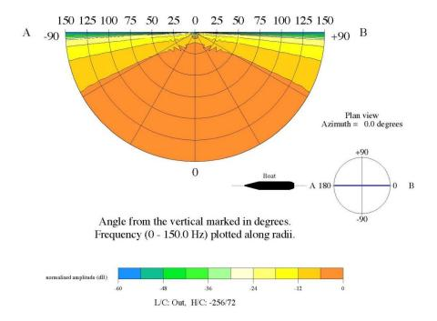
Source Directivity Plot - azimuth : 0.0 degrees - array SeaScan\_2x880\_3M
