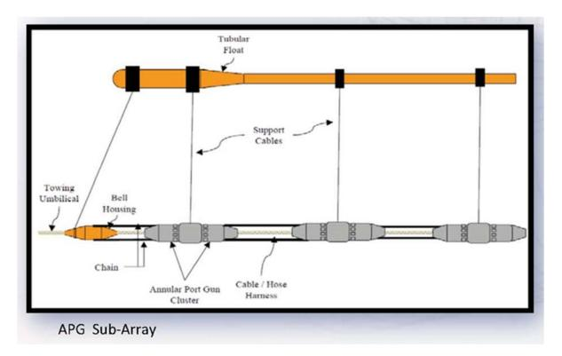
Figure 1-6. APG Sub-Array Sound Source (Example)
