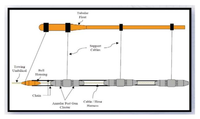
Figure 1-6. APG Sub-Array Sound Source (Example)
