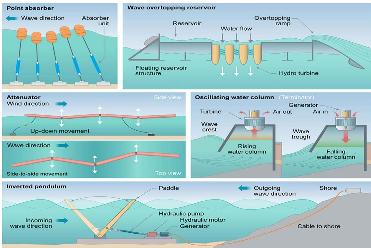
**Figure 1-1. Wave energy conversion device topologies**
