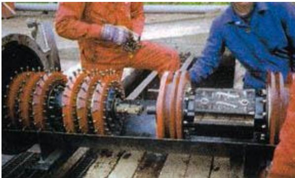
Figure R.12. Pigging operations remove buildup from pipeline and prevent corrosion
