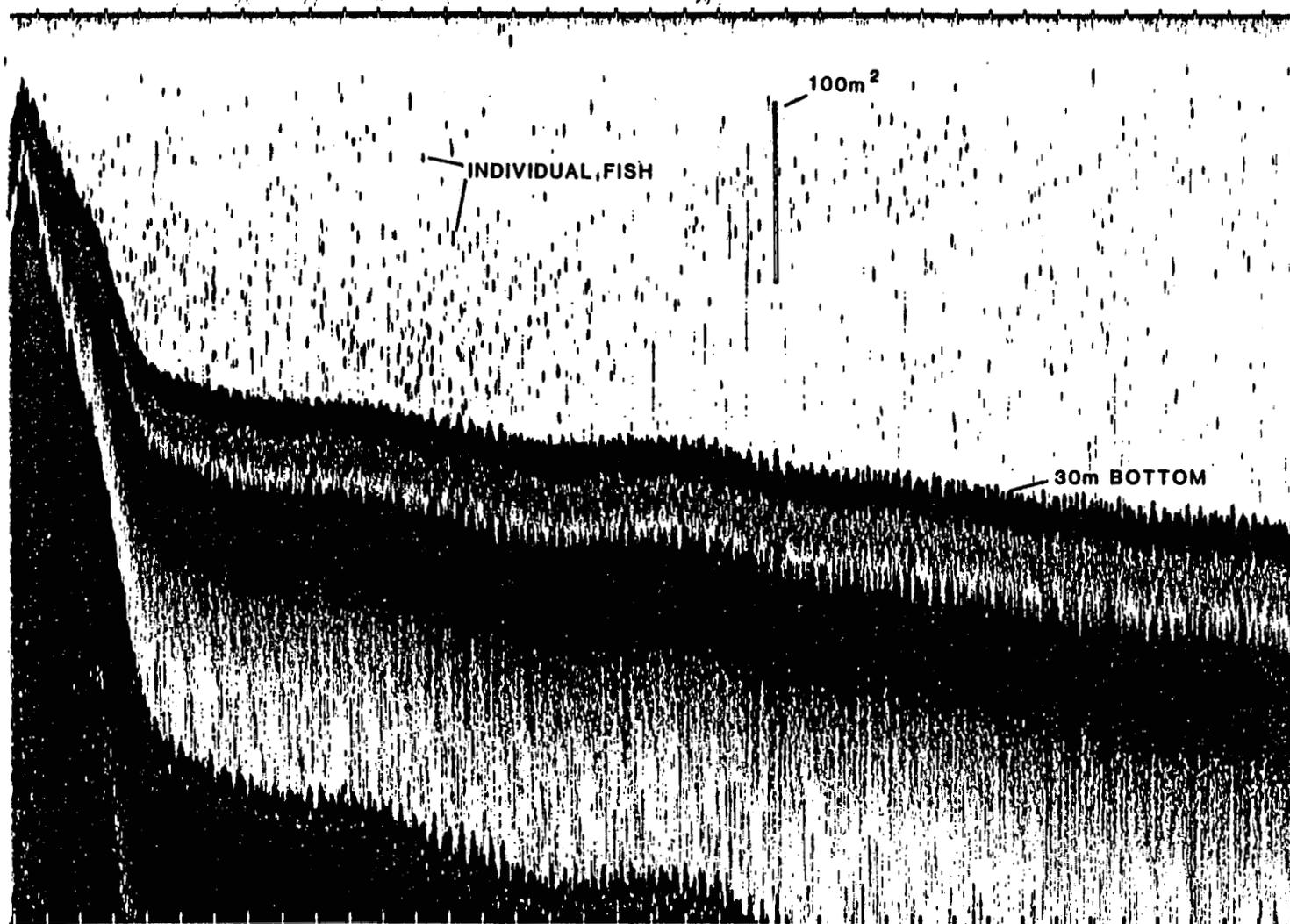
Figure 5.9. Hydroacoustic echogram recorded near station 'a' on survey No. 10 northwest of Cape Thompson (see Figs. 5.2 and 5.8). Fish densities near the bottom and in mid-water averaged  $1.6 \text{ g/m}^3$ .
