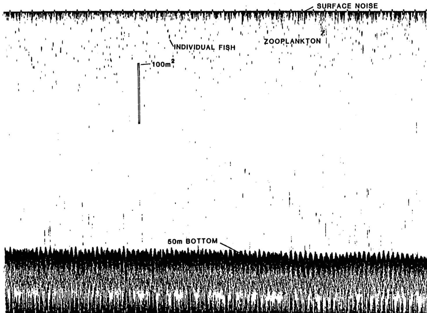
Figure 5.10. Hydroacoustic echogram recorded near station 'c' on survey No. 10 northwest of Cape Thompson (see Figs. 5.2 and 5.8). Note the concentrations of zooplankton and fish ( $<0.2 \text{ g/m}^3$ ) pushed towards the surface by upwelling in this convergent zone.
