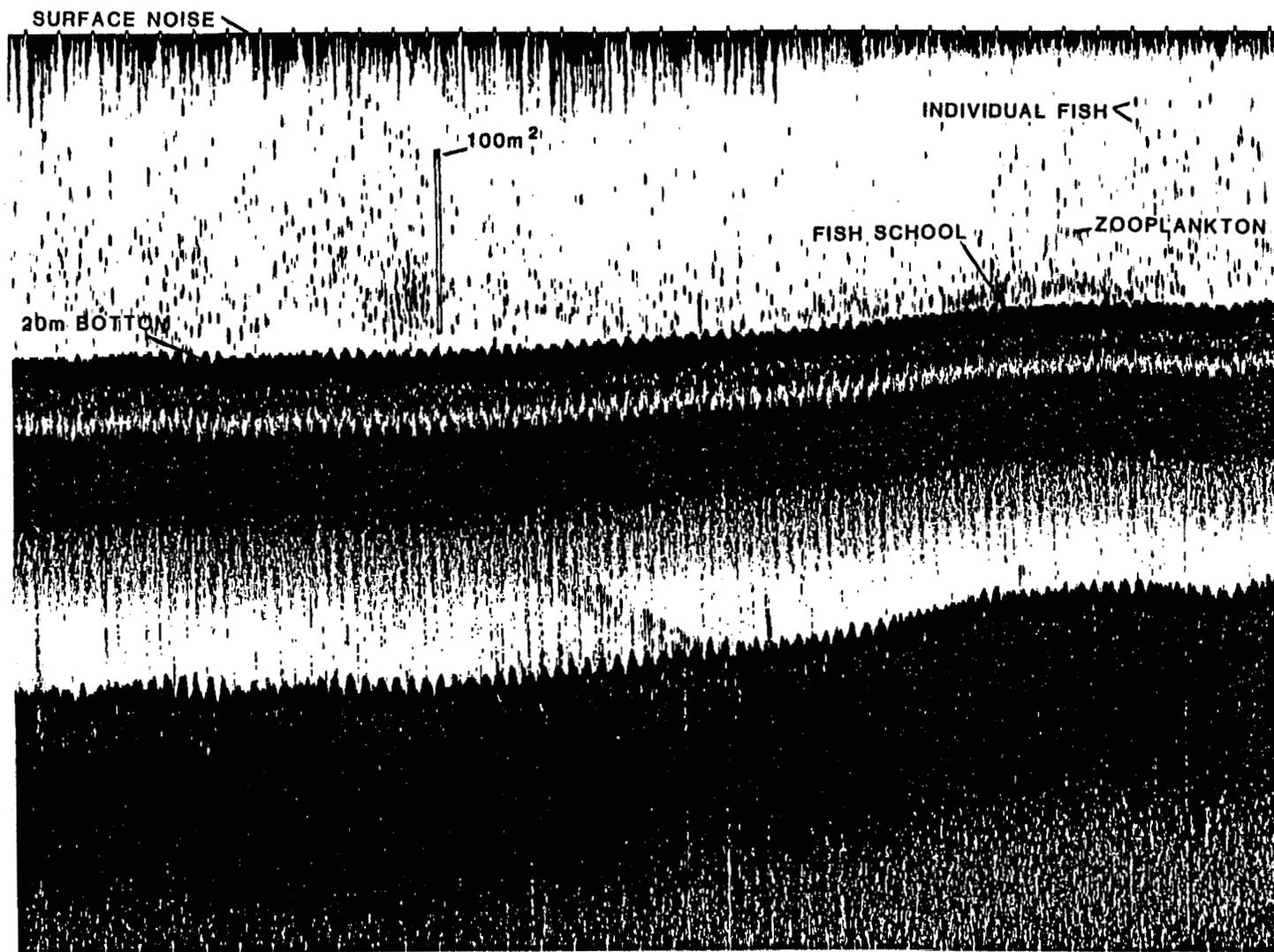
Figure 5.13. Hydroacoustic echogram recorded between waypoints 'b' and 'c' on coastal survey No. 11 (see Figs. 5.2 and 5.12). Fish densities at the indicated school were  $193 \text{ g/m}^3$ .
