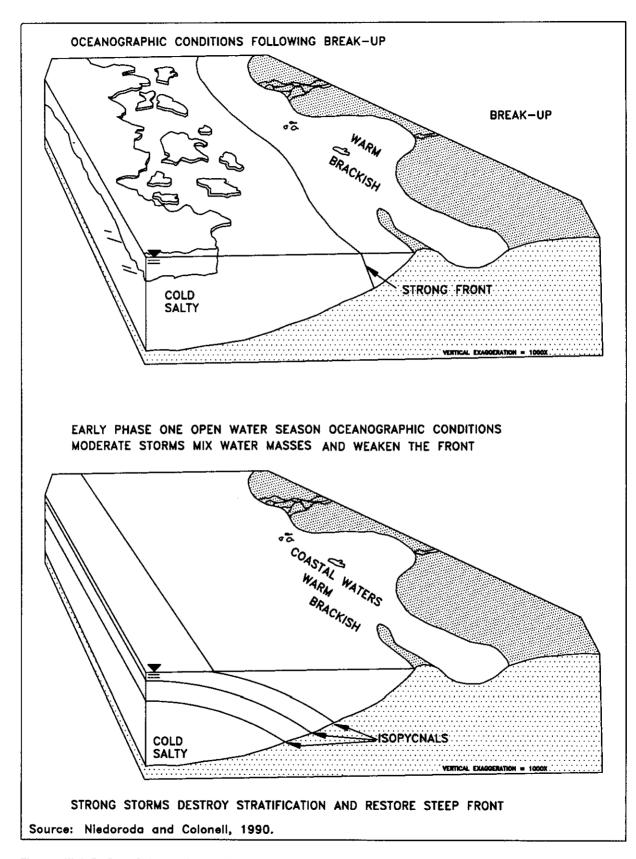
Figure III.A.3-2a Schematic of Nearshore Circulation
