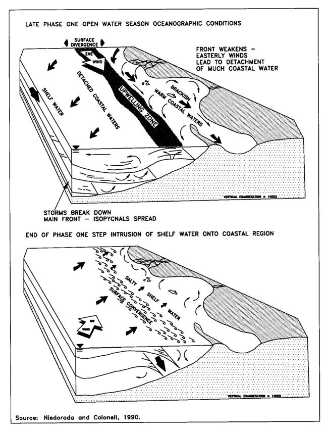
Figure III.A.3-2b Schematic of Nearshore Circulation
