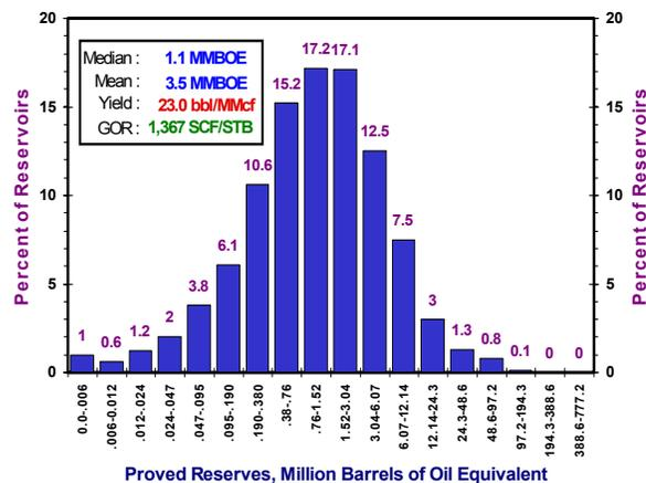
Figure 31. Reservoir-size distribution, 1,671 proved combination reservoirs.
