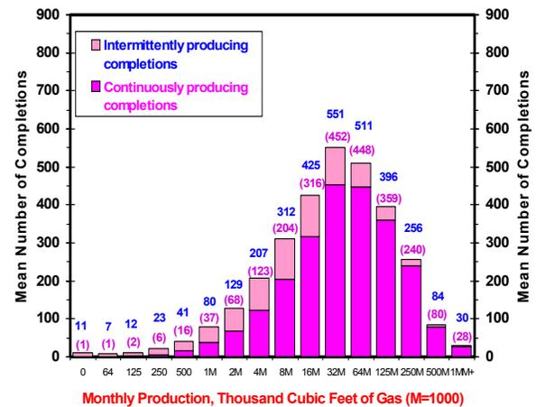
Figure 35. Monthly distribution of gas production, 3,075 completions, (2,381 continuously producing completions).
