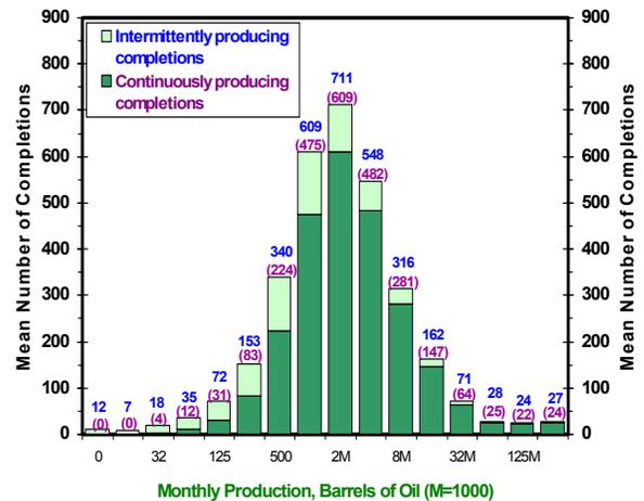
Figure 34. Monthly distribution of oil production, 3,133 completions, (2,483 continuously producing completions).
