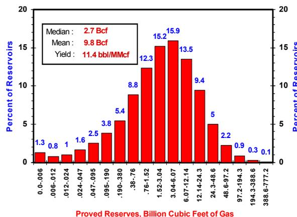
Figure 33. Reservoir-size distribution, 13,703 proved gas reservoirs.
