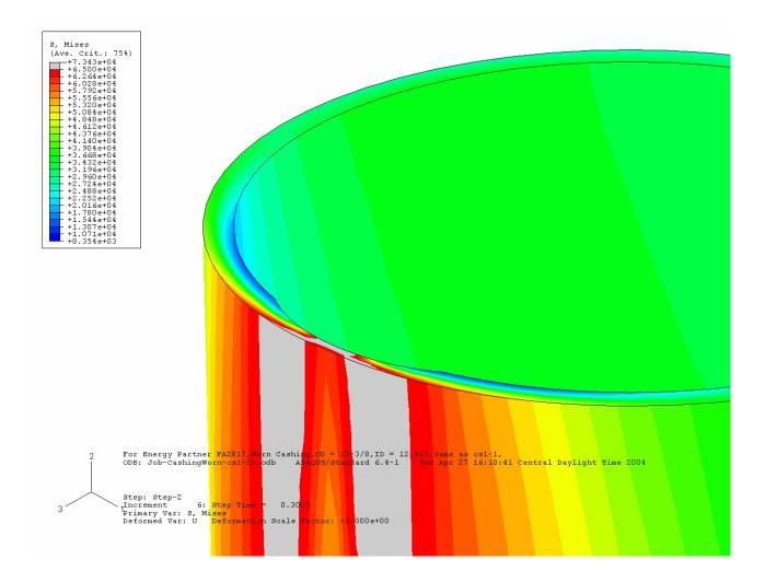
Internal pressure of 2,300 psi produced through-wall yielding of the worn casing joint [From T. H. Hill].
