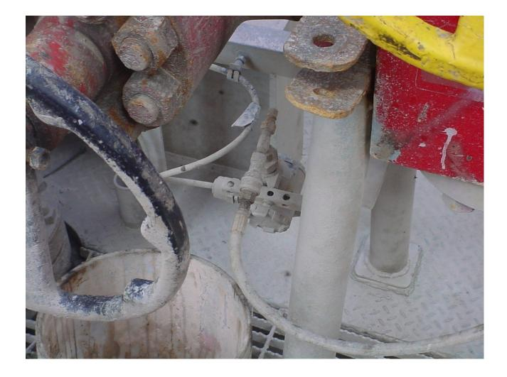
Hydraulic line to driller's console gauges and reservoir, after incident.
