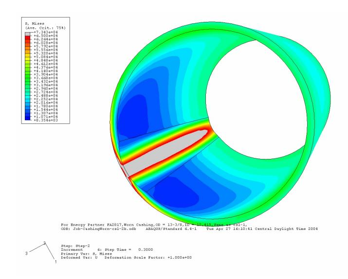
Stress distribution along the inside surface of the worn casing [From T. H. Hill].
