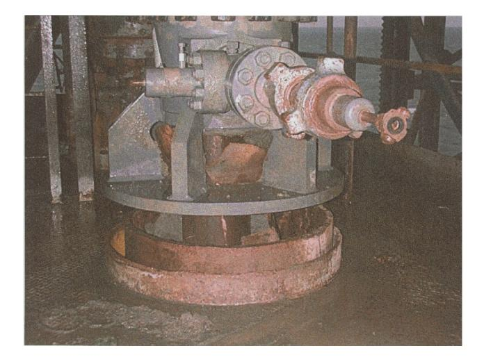
Wellhead: After the incident, showing parted casing.
