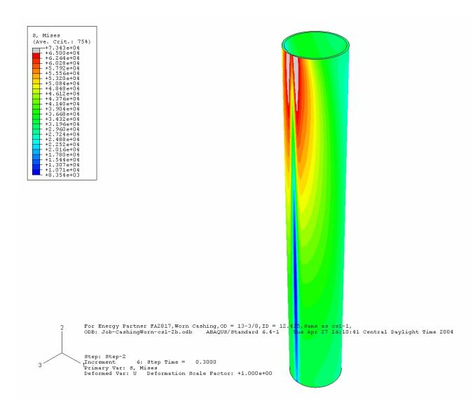
Stress distribution along the outside surface of the worn casing [From T. H. Hill].
