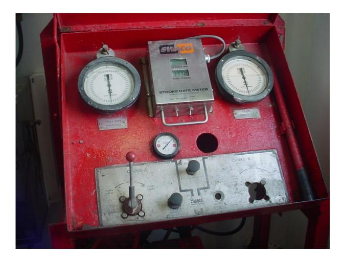
Driller's console gauges.
