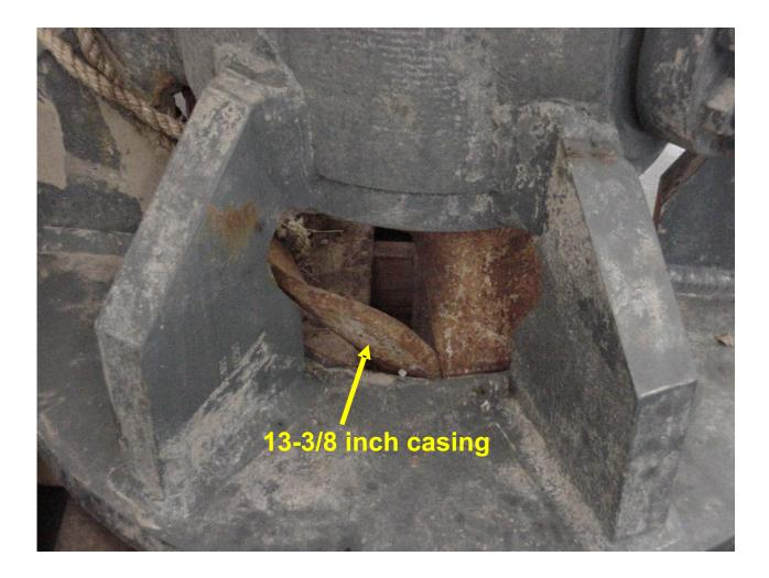
Damaged 13 3/8 inch slip-on wellhead (SOW) and casing.
