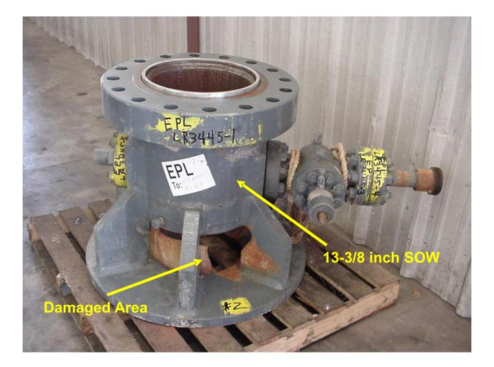
Damaged SOW and top of 13 3/8 inch casing.
