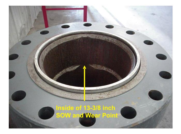
Worn and damaged 13 3/8 inch SOW.
