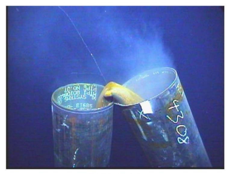
Pipe failure by bending.
