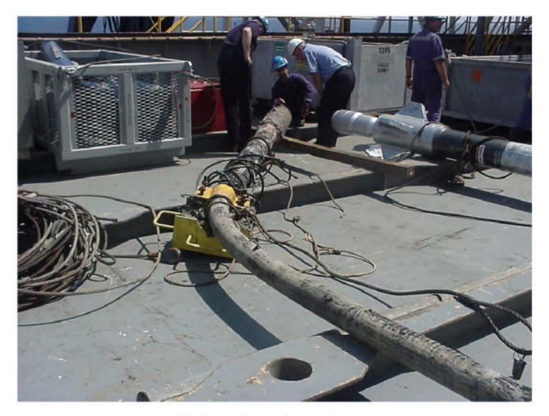
Drill pipe bending below running tool.
