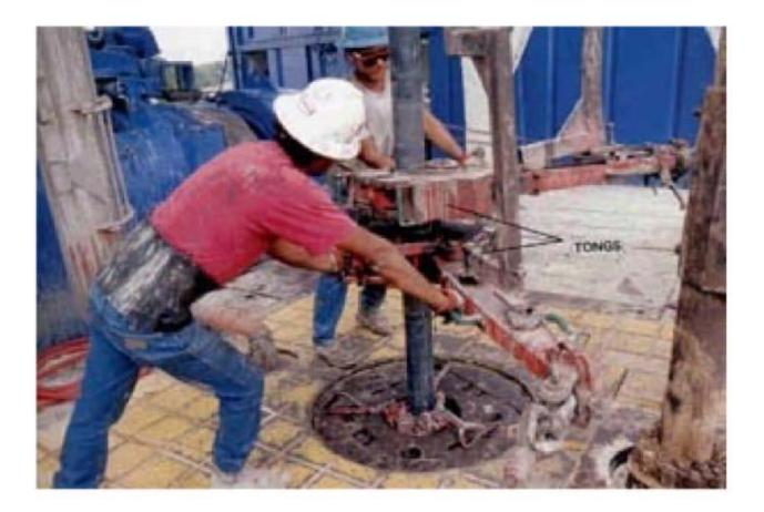
View of drill pipe in rotary slips.
