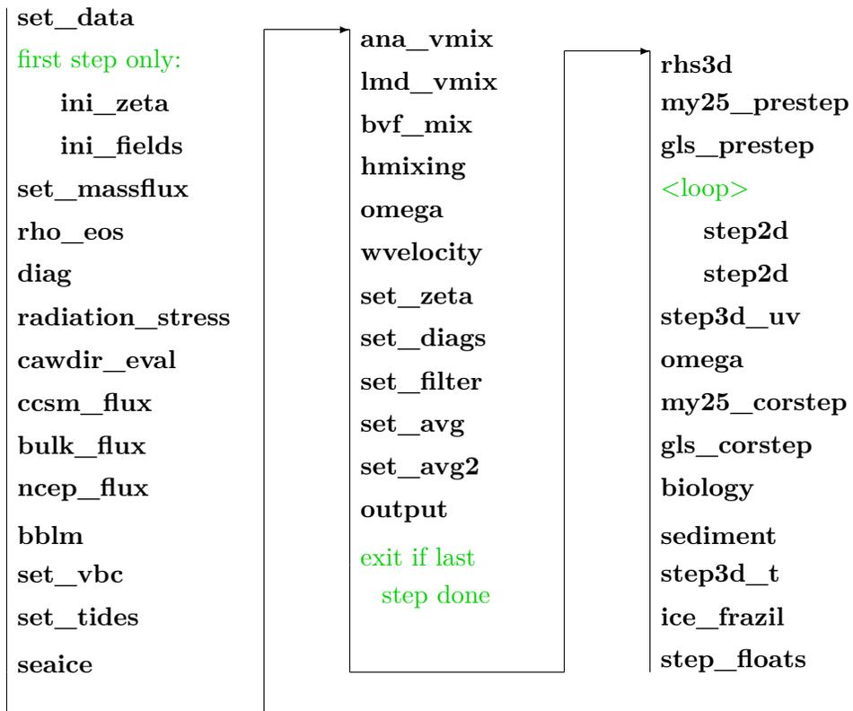
Figure 11: Flow chart of the model main program.
