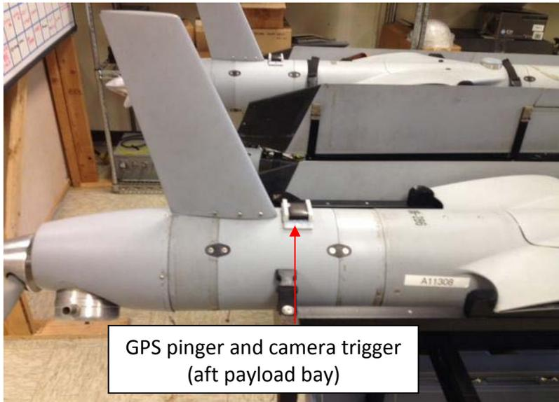
Figure 7: AFT payloads in the ScanEagle®
