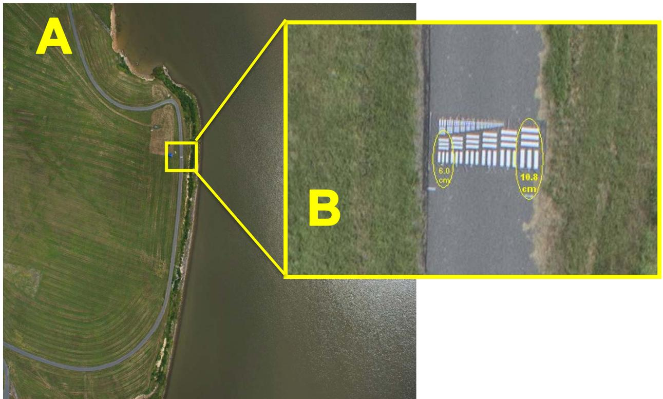
Figure 8. Image A was taken from the UAS during the test flight in Dahlgren, VA at 1050 ft AGL and 60 kts ground speed. Image B shows the calibration target at 300% zoom, with circles around the 6 cm wide and 10.8 cm wide calibration tribars.
