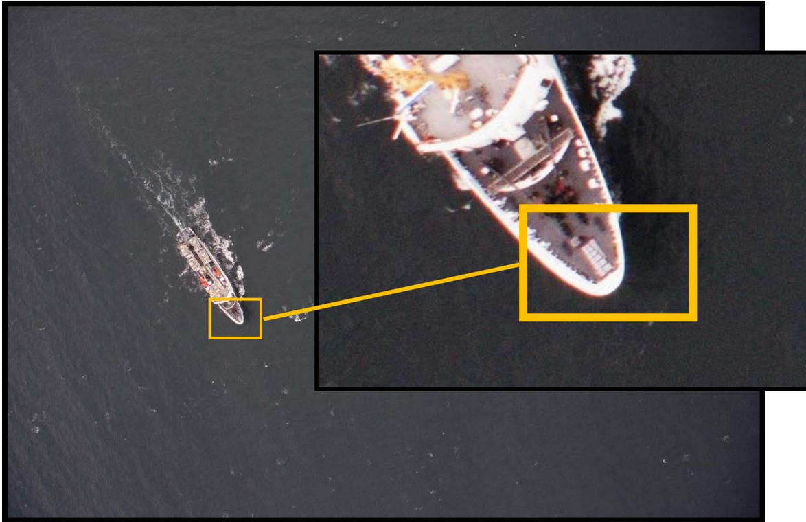
Figure 13. Calibration target on the NOAA Ship *Fairweather*, photographed from the UAV at 997 ft MSL. The yellow boxes indicate the location of the calibration target and a zoomed insert of the target.
