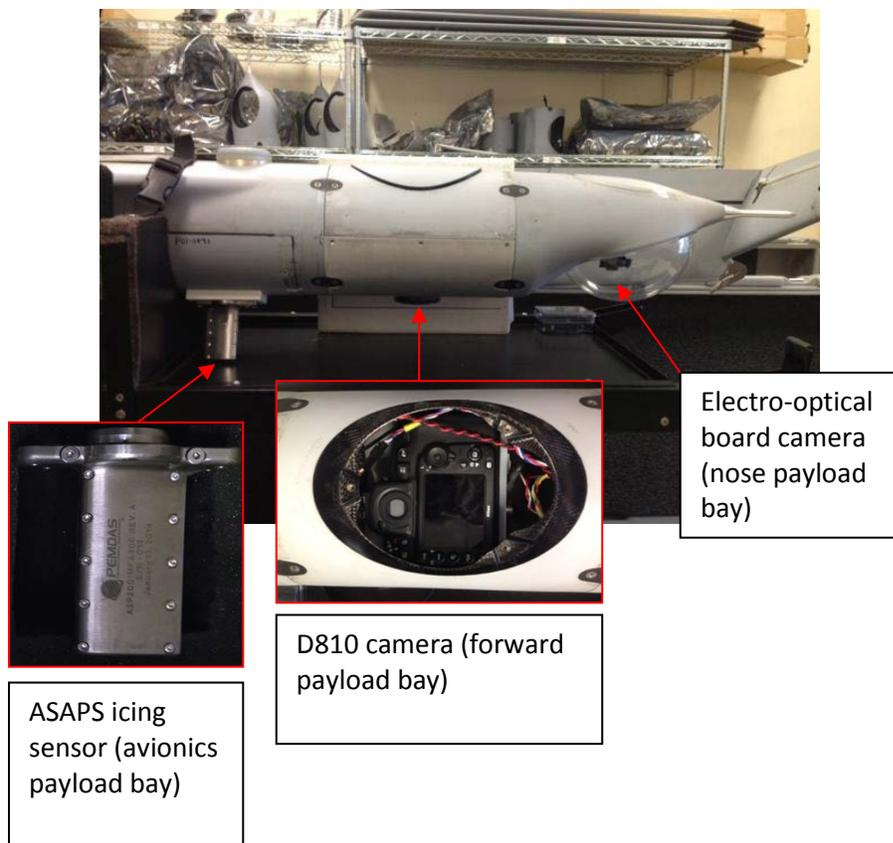
Figure 6: Forward payloads in the ScanEagle®
