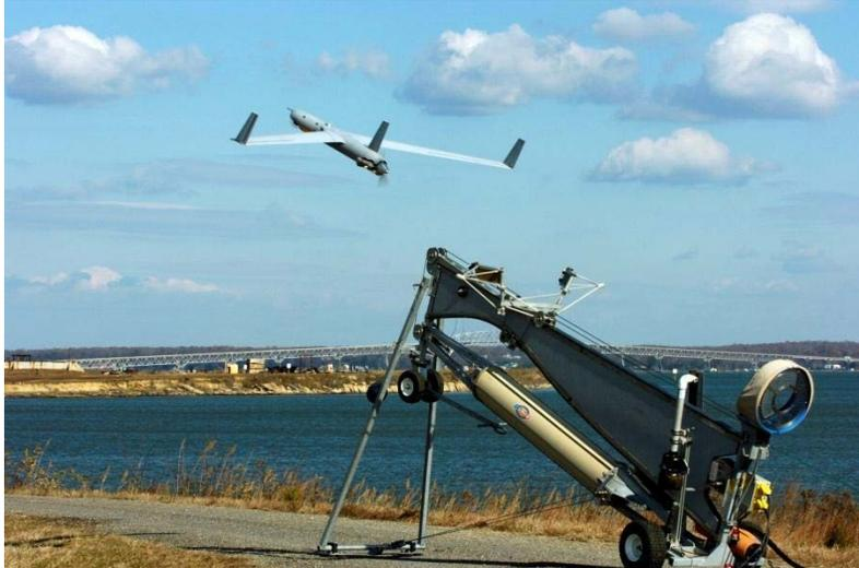
Figure 3. ScanEagle® on launch at Naval Surface Warfare Center – Dahlgren Division
