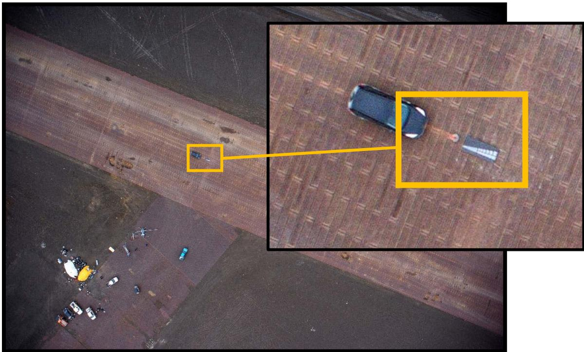
Figure 12. Calibration target at the NARL field site. Yellow boxes indicate the location of the calibration target and a zoomed insert of the target.
