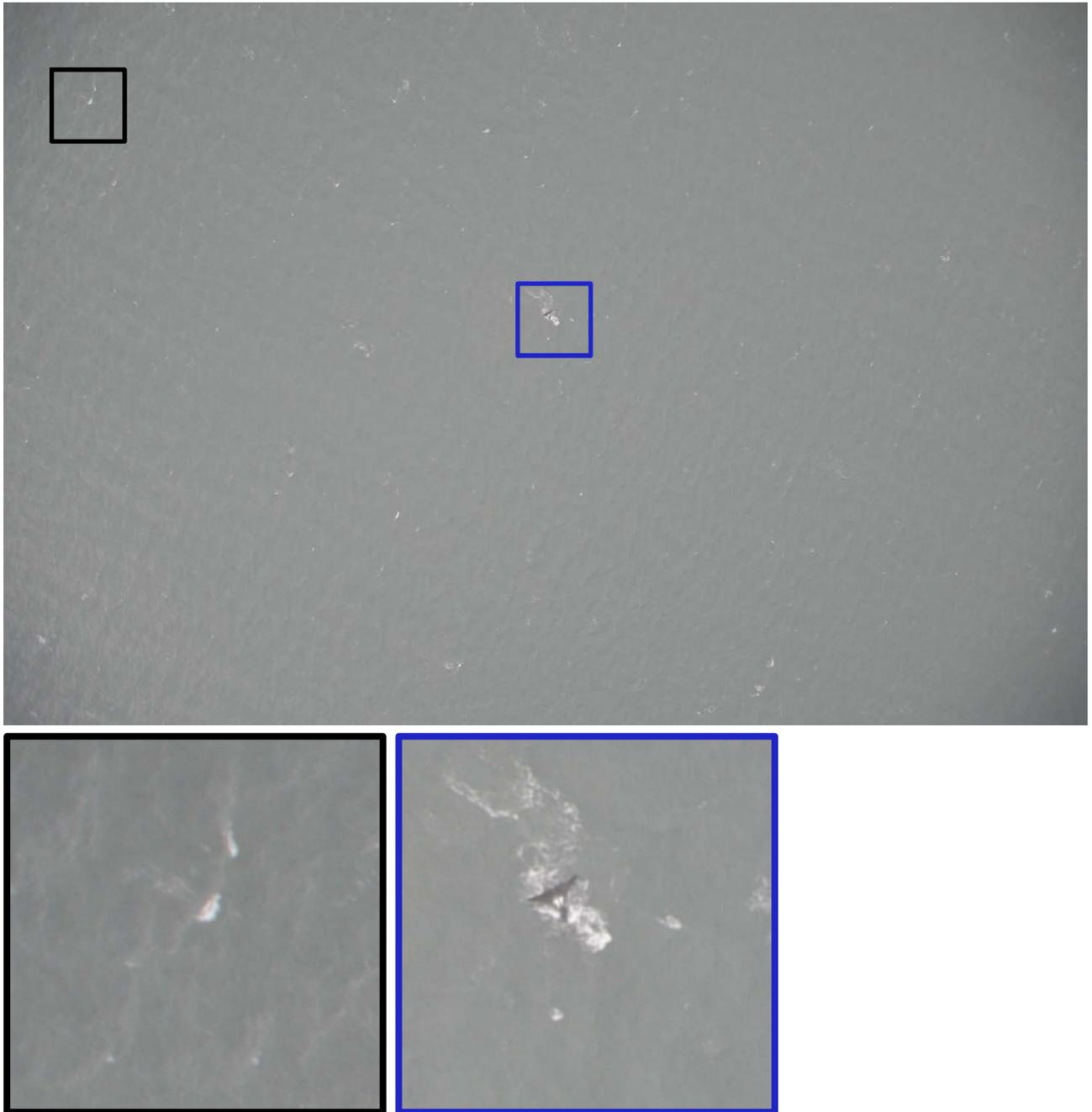
Figure 16: Top: The Brainlike, Inc.® AMMD “alert map” showing the original image with “chips” (detections), outlined in blue and black boxes. Bottom: Corresponding blue and black “chips”. The black chip (bottom left) is a false positive detection and the blue chip is a true positive detection of the dorsal fluke of a diving bowhead whale.
