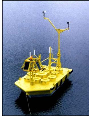
**Figure 3-8b. 6-meter Boat-shaped Hull Buoy**
