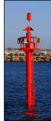
**Figure 3-8c. Spar Buoy**
