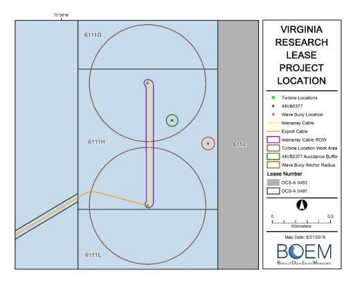
Figure 4. Closeup of project offshore elements, including buoy location. Work occurring around the north WTG will avoid site 44BV0377 (dark green dot) by 500m (dark green circle.
