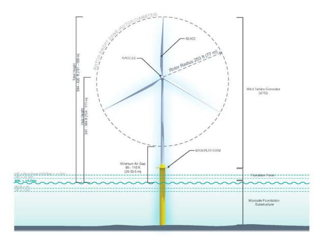
Figure 3. Conceptual rendering of the proposed WTG and foundation.
