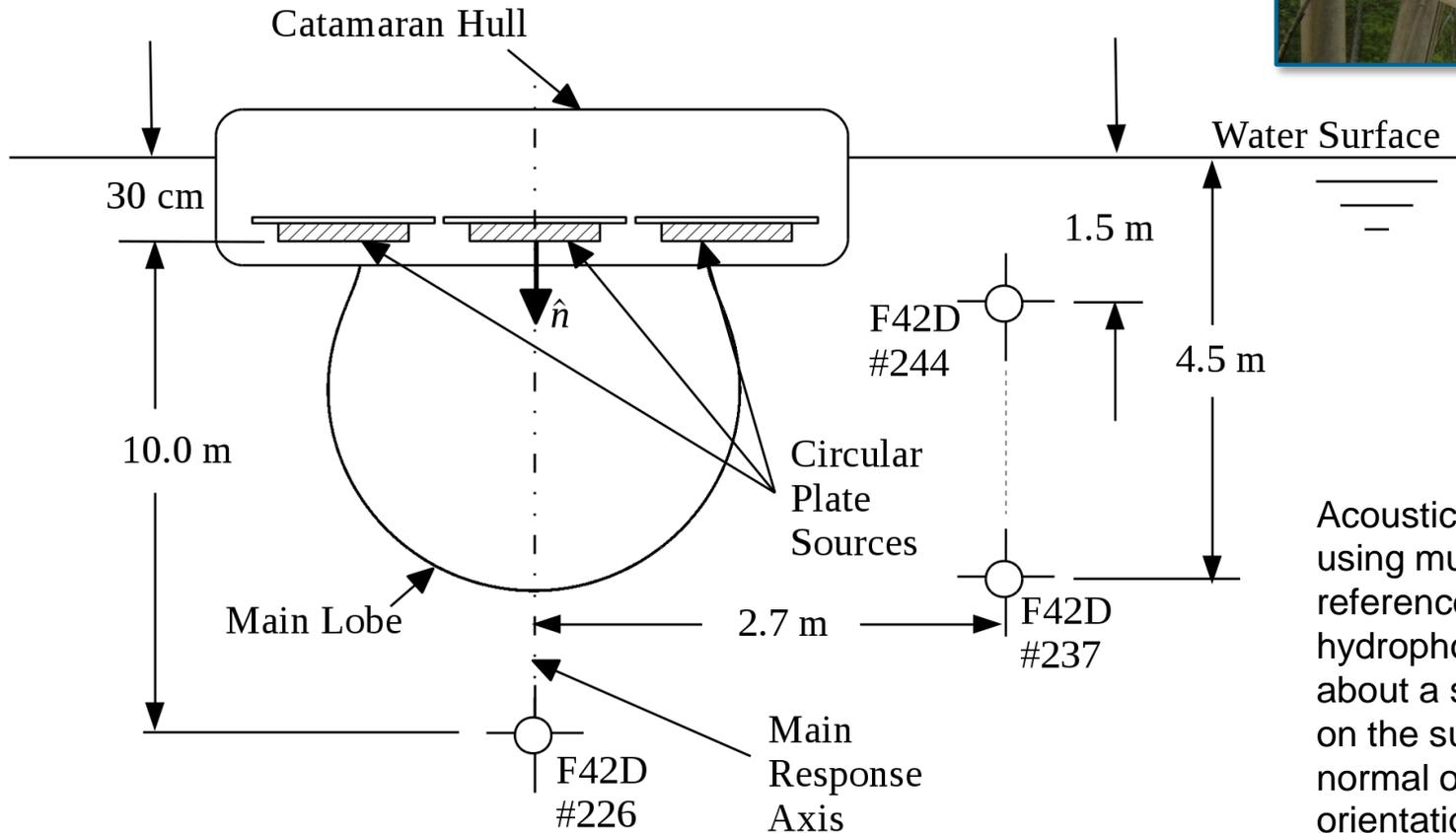
Acoustic data collected using multiple calibrated reference standard hydrophones distributed about a source deployed on the surface in its normal operating orientation
